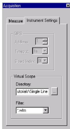
**Figure 4-2: Setting the virtual scope options**
