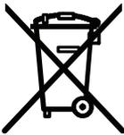
The symbol shown to the left indicates that this product complies with the European Union's requirements according to Directive 2002/96/EC on waste electrical and electronic equipment (WEEE). For information about recycling options, check the Support/Service section of the Tektronix Web site ([www.tektronix.com](http://www.tektronix.com)).
