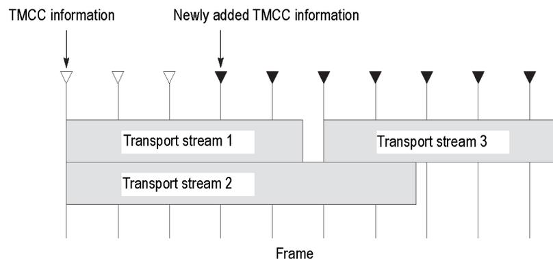
This illustration shows the placement of the new TMCC information and the transport stream 3 when they are multiplexed after the transport stream 1. The
