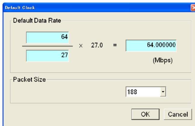
**Default Data Rate:** Overwrites the scanned bit rate value of the stream file.
