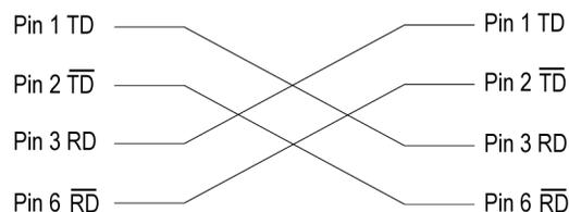
**Figure 3-35: Pin connections for a crossover Ethernet cable**
