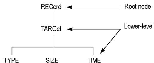
**Figure 3-42: Example of SCPI subsystem hierarchy tree**
