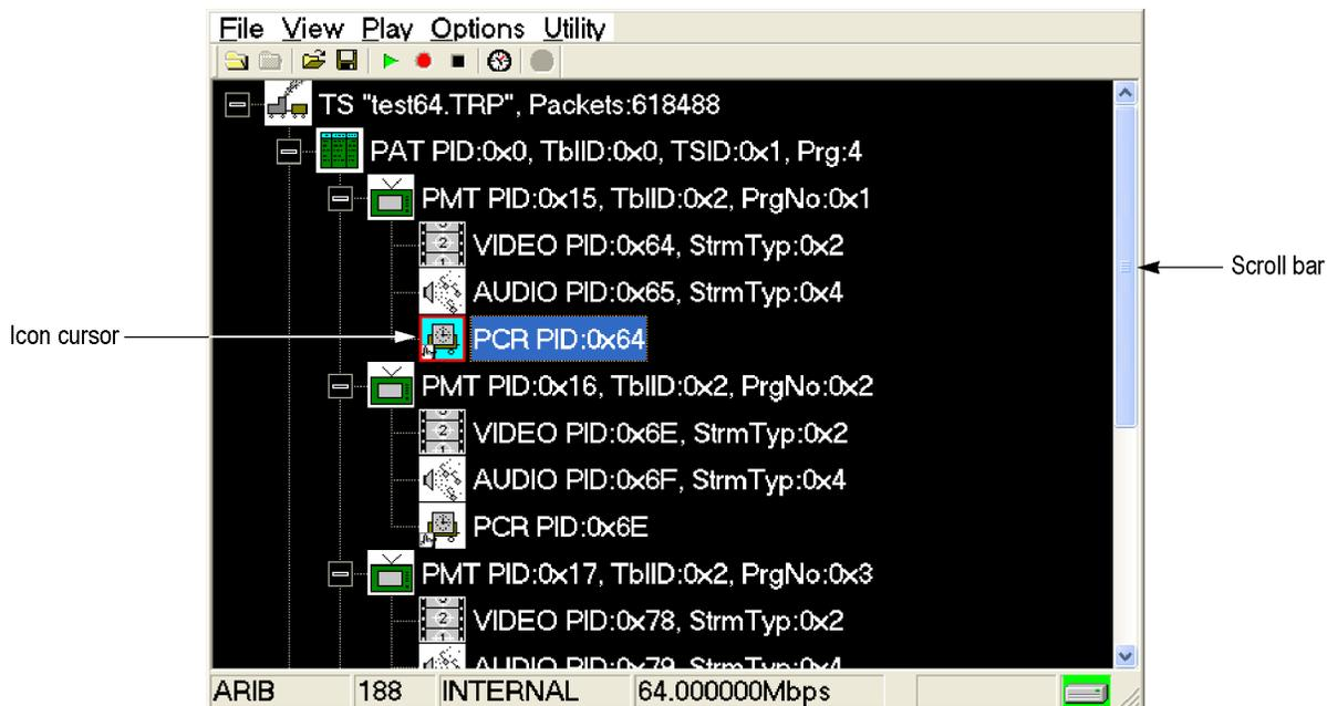
Figure 3-27: Example of the hierarchy display
