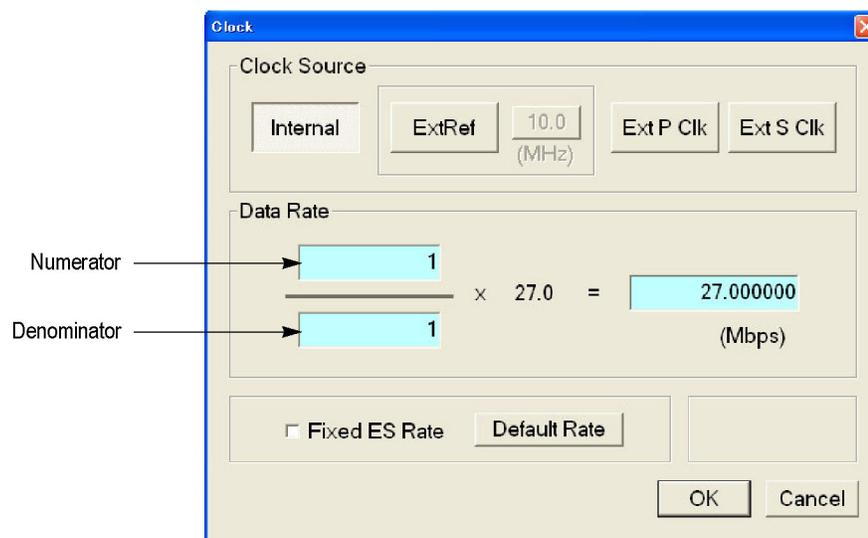
**Figure 3-2: Clock dialog box for Option Interface**
