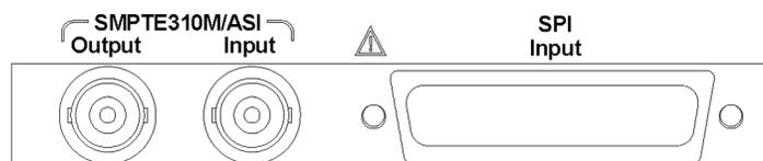
**Figure 2-10: SMPTE310M/ASI/SPI interface**
