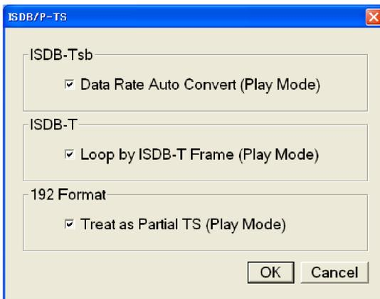
**Data Rate Auto Convert (Play Mode):** Sets whether the clock rate is set automatically when the ISDB-TSB file is loaded. When selected, the clock rate is automatically set to  $(2048/1701) \times 27$  MHz and the elementary stream rate becomes constant regardless of the Fixed ES Rate setting.
