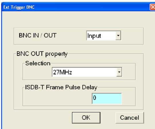
**BNC IN/OUT:** Sets whether to use the rear-panel Trig In/Out connector as a trigger signal input or a reference clock/ISDB-T frame clock signal output. You can select Input or Output. For Input, the Trig In/Out connector can be used to input an external trigger event. For Output, the Trig In/Out connector can be used to output a 27 MHz reference clock or an ISDB-T frame pulse signal. Use the Selection list box to select which signal is output from the connector.
