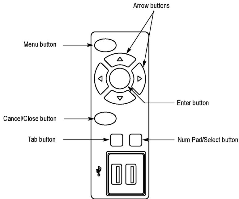
**Figure 2-11: Front panel showing the menu controls**
