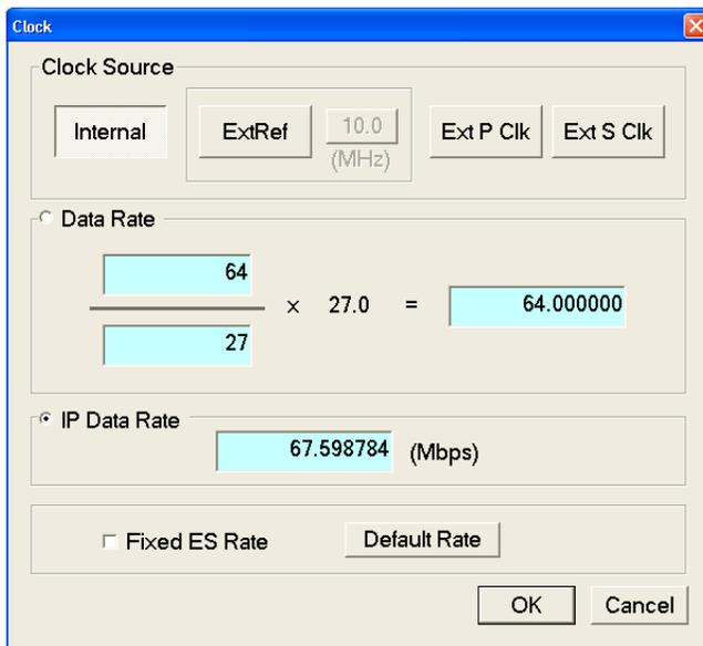
Figure 3-3: Clock dialog box for IP Interface
