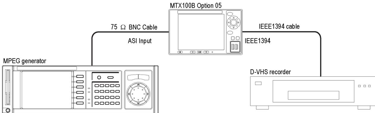
Figure 3-50: Connection example for ASI to IEEE1394 conversion
