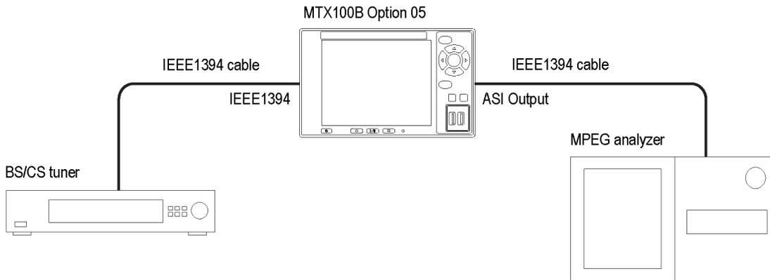
Figure 3-51: Connection example for IEEE1394 to ASI conversion
