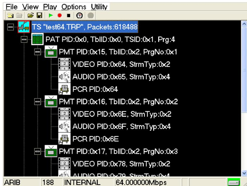
Figure 2-15: Hierarchy view of the transport stream file
