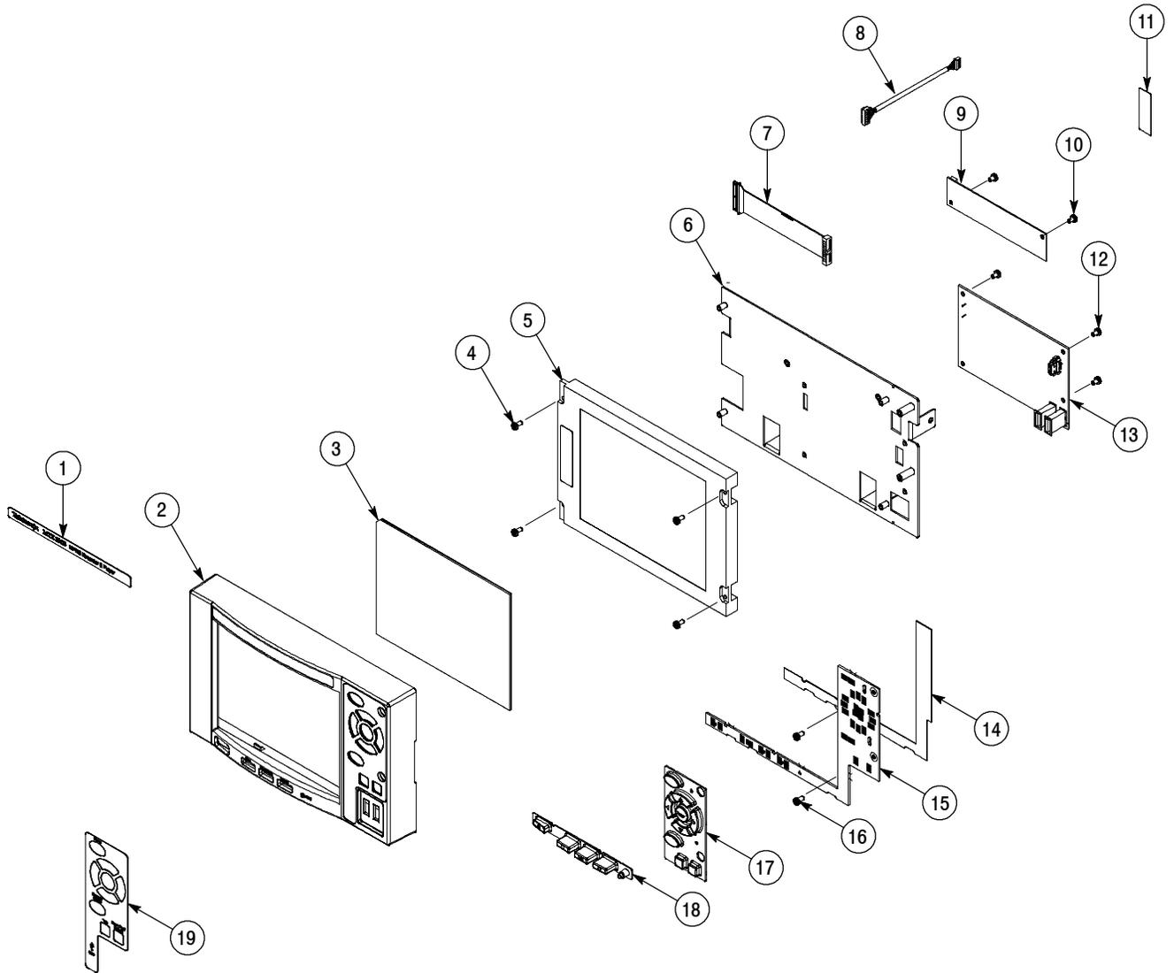
Figure 8-4: Front panel unit
