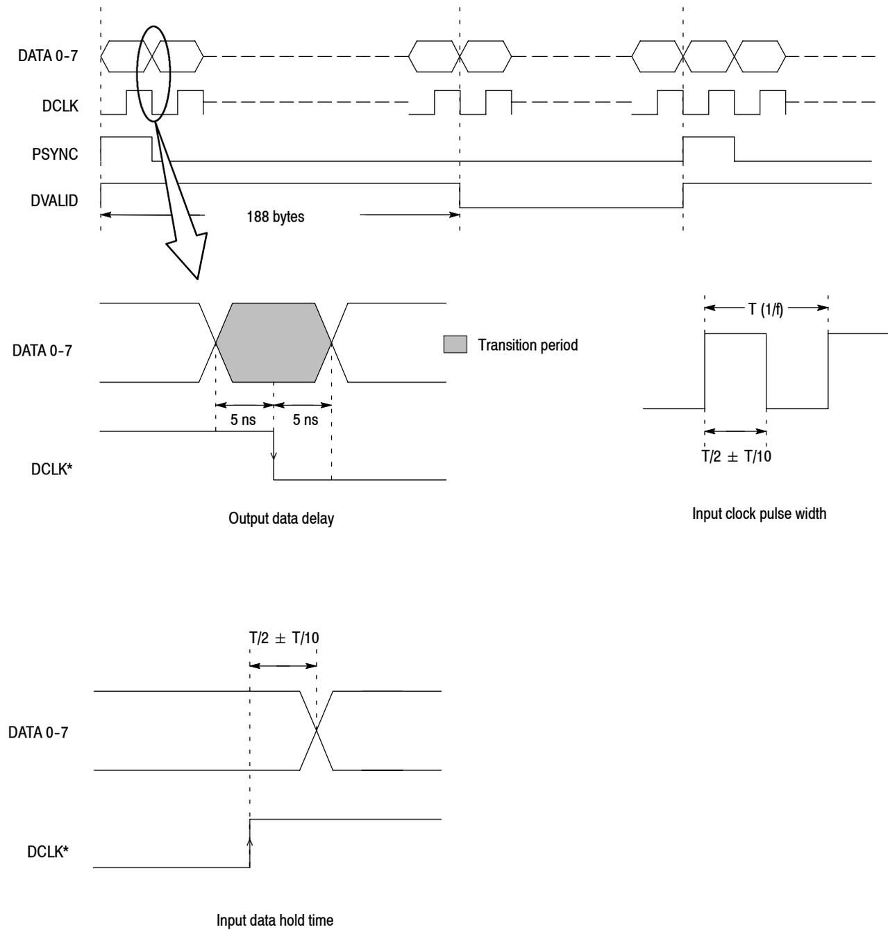
**Figure 1-1: Timing diagram of the SPI interface**
