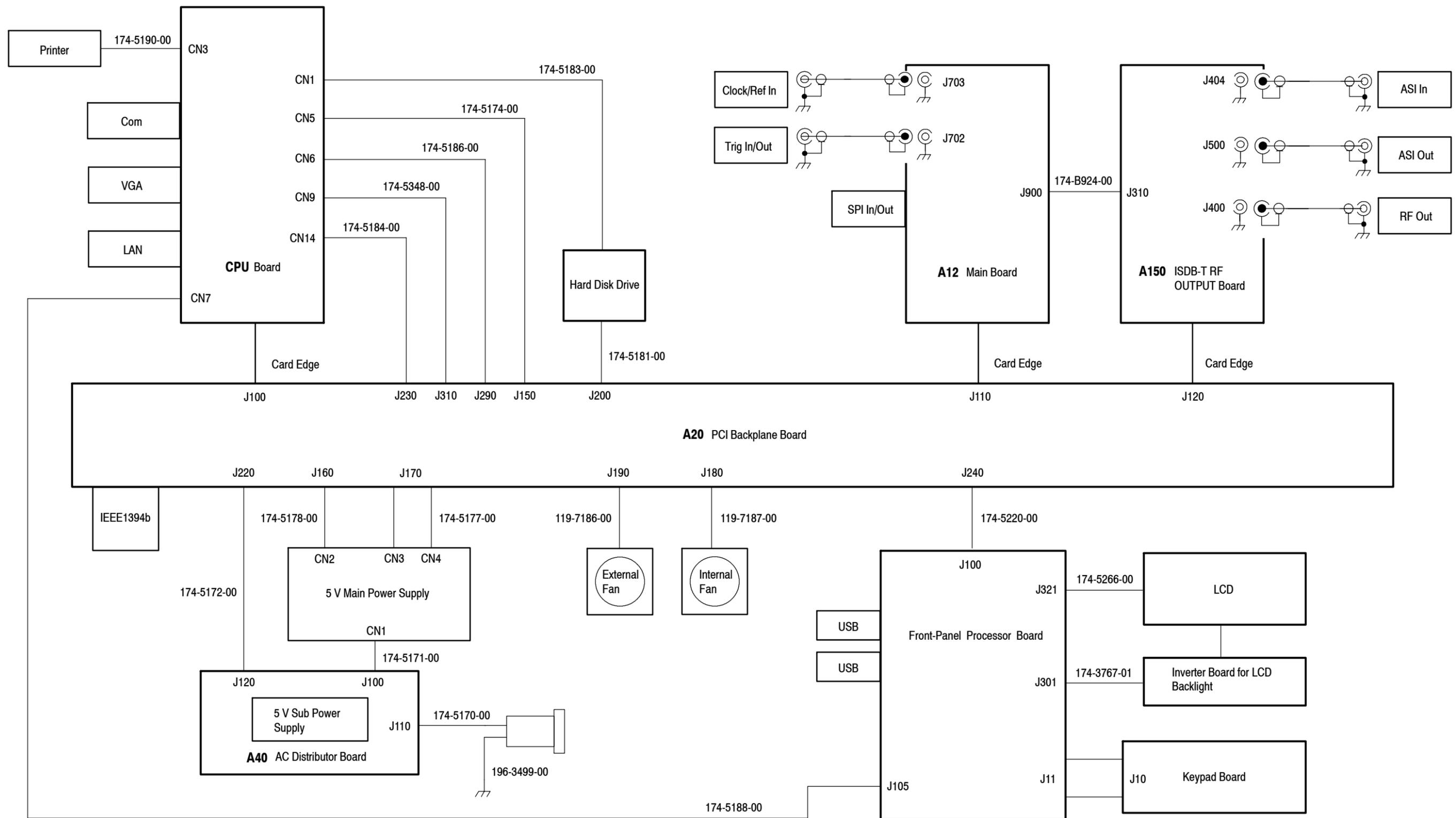
Figure 7-2: RTX100B interconnect diagram
