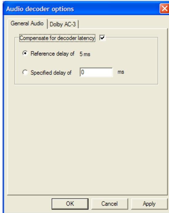
With Compensate for decoder latency selected, a reference delay appropriate for the decoder in use is automatically available. If you want to specify a different delay, enter the value in the Specified delay field and select the option.
