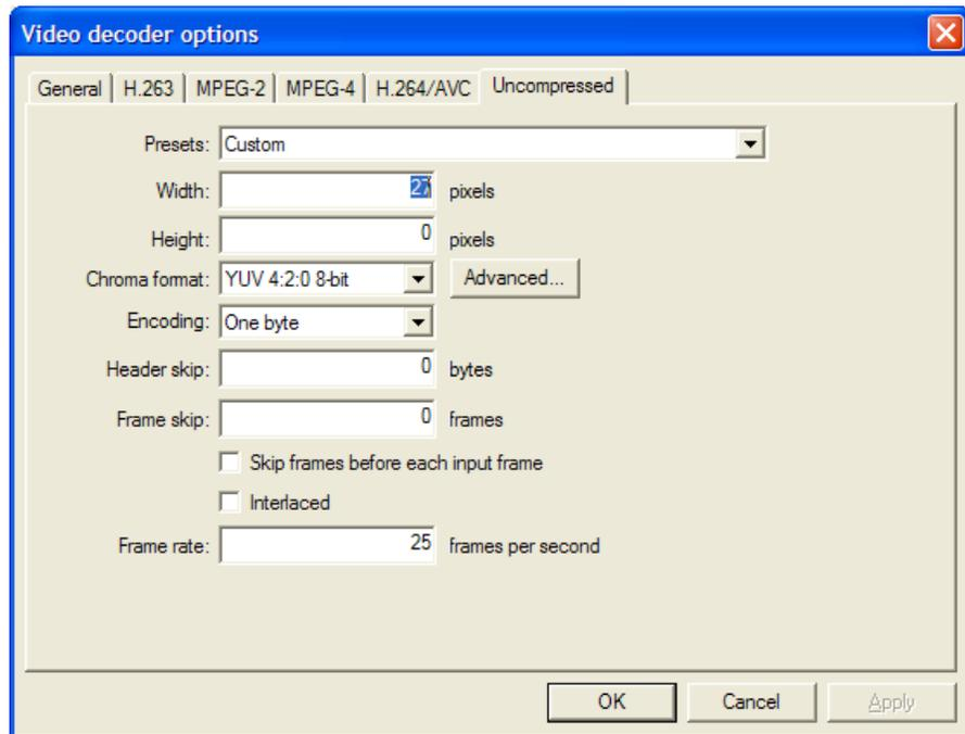
**Presets (Width and Height).** If there are numbers in the filename that could indicate the frame size, the MTS4CC will attempt to read these and offer these in the Width and Height fields shown in the previous figure. The correct values can be entered or selected using the drop-down list:
