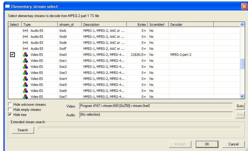
**Search (Extended stream search).** For some standards, the total size of the stream is indicated in the container file - for example, MPEG-4. In this case, the size of the elementary stream is shown.
