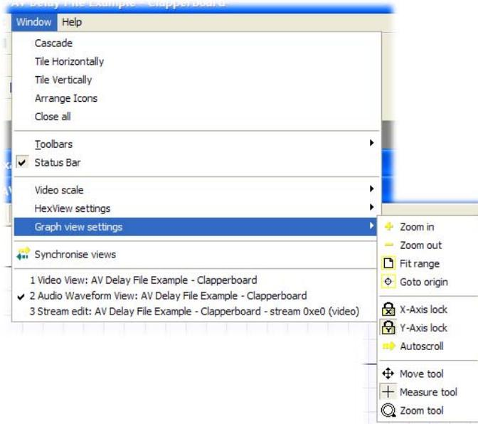
The Graph view menu has ten options, which control how the data appears on the Buffer analysis graph. These options are described in the following table:
