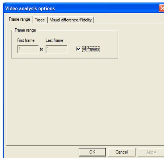
**All frames.** This option is the default and calculates the sequence statistics from the start of the sequence until the current frame.
