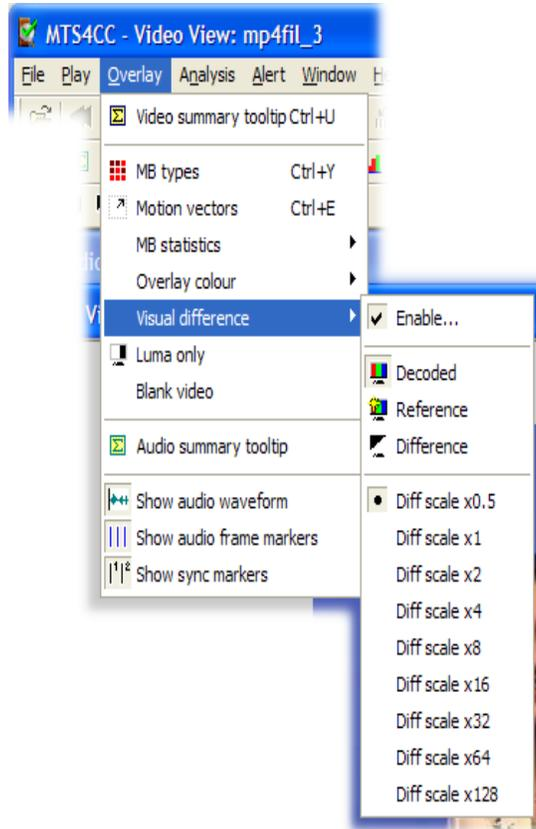
This menu option enables the visual difference video display; this uses an uncompressed video reference file to show a video view of any of the following:
