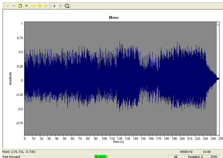
The gray background is due to the density of marked-off frames; when the zoom out icon is used, the spacing between the frame marking increases and the shape of the waveform becomes more easily discernible (see the following figure). At each frame marker, the frame type and number is shown.
