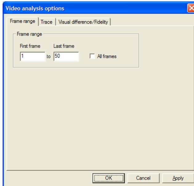
When a range of frames has been set, the Frame range item on the MB statistics menu changes, with a check mark to indicate a range of frames has been set:
