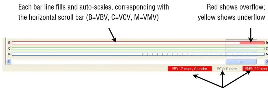
Each buffer item changes to red or yellow if there has been any overflow/underflow, and the number indicates in how many frames there is non-conformance. If there is both overflow and underflow, the color is red.
