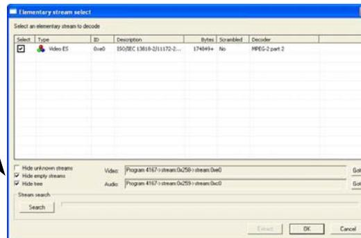
When a container file is loaded, the MTS4CC automatically opens the Elementary stream select window (as shown in the preceding figure), which lists all streams, audio and video. The streams can be browsed, individually selected for analysis with your choice of decoder, and either immediately played and analyzed within the MTS4CC or extracted and saved to a file before going on to play/analyze them.
