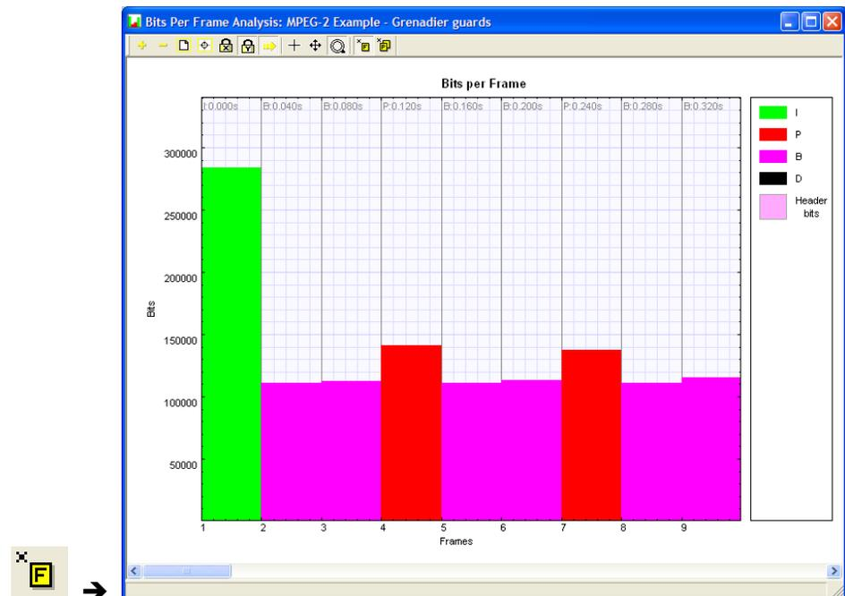
The Picture units toolbar button also displays the total bits per frame, but, in the case of interlaced pictures, each frame contains two picture fields:
