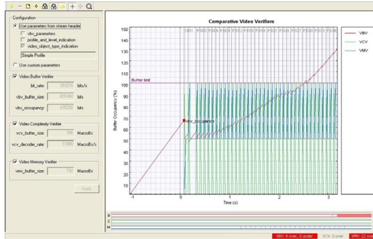
**Buffer analysis controls: MPEG-4 and MPEG-2.**
