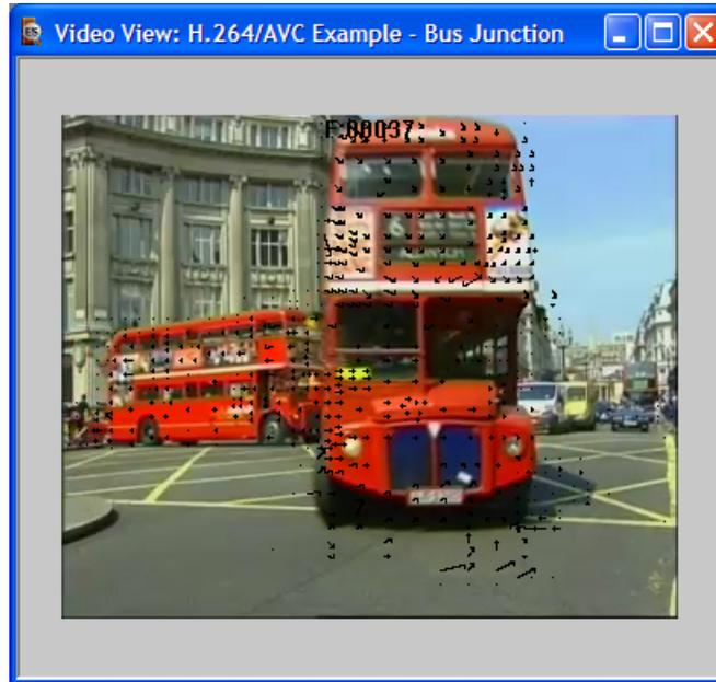
The motion vectors are plotted to the length of that actually used by the decoder.
