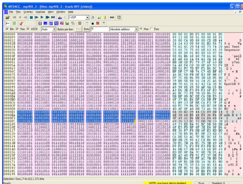
This opens the current video file in a hex viewer, which shows the data in binary, hexadecimal, and ASCII data (in any combination of the three).
