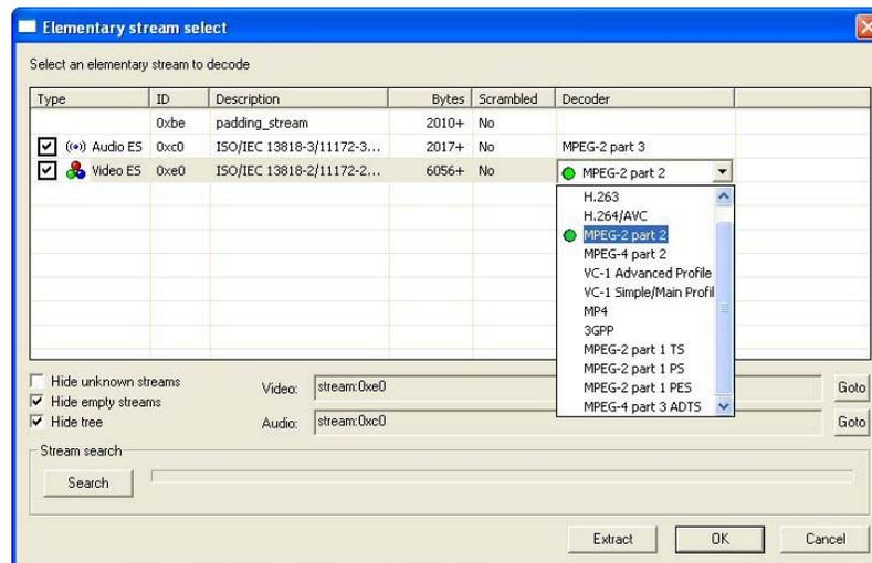
Selecting a different decoder forces the MTS4CC to use that decoder for this track/Elementary Stream.
