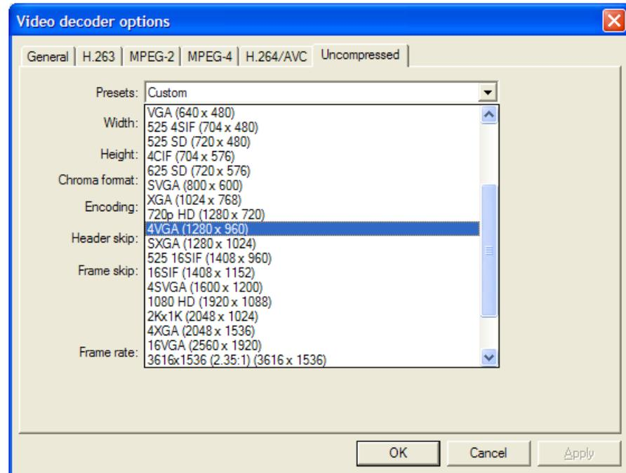
**Chroma format.** This control specifies the color model and format for the uncompressed video data. The combo provides several common combinations, including 8-bit YUV 4:2:0, 8-bit YUV 4:2:2, 8-bit YUV 4:4:4, 8-bit RGB and 8-bit grayscale. Select an entry from the list to use one of these common formats. Other formats can be specified by choosing the Custom entry in the list - this will open the Image format dialog.
