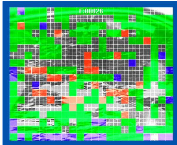
This example is a B-VOP of an MPEG-4 Advanced Simple Profile stream.
