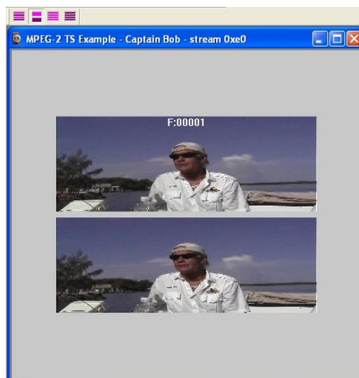
**Top-field view.** Only the top-field image data is displayed. For field coded MacroBlocks, the MB tooltip and overlays show data relevant to the top field. For frame coded MacroBlocks, the MB tooltip and overlays show data relevant to the frame.
