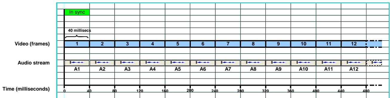
The preceding illustration shows video being decoded at a display rate of one frame every 40 milliseconds. Audio plays, unbroken, at the same rate as the video.
