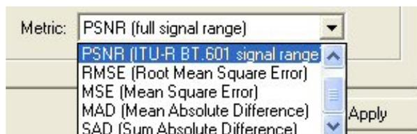
The objective fidelity metrics provided by MTS4CC measure the degradation of the decoded image with respect to a reference image. The metric is evaluated independently for each image plane in the color space dictated by the video decoder (typically YUV).
