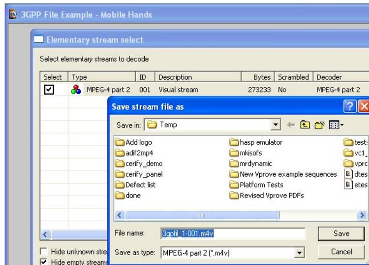
In this example, the video elementary stream from E-City.mp4 video track 1 is being saved to an .m4v file: the -001 (for track 1) and .m4v are automatically added by MTS4CC (because MTS4CC knows this is a 3GPP file), although any file name and extension can be entered.
