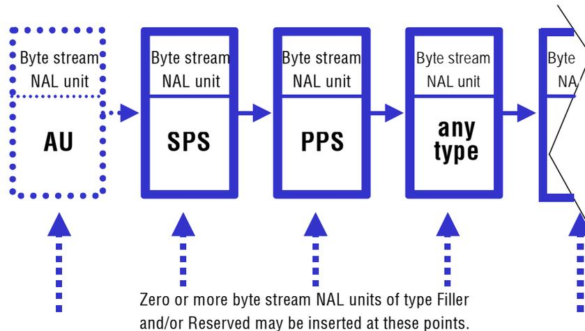
For example, if the bitstream does not contain the optional items at the start then the first six bytes in an Extended profile byte stream file will be: 00 00 00 01 67 58 (all values in hexadecimal).
