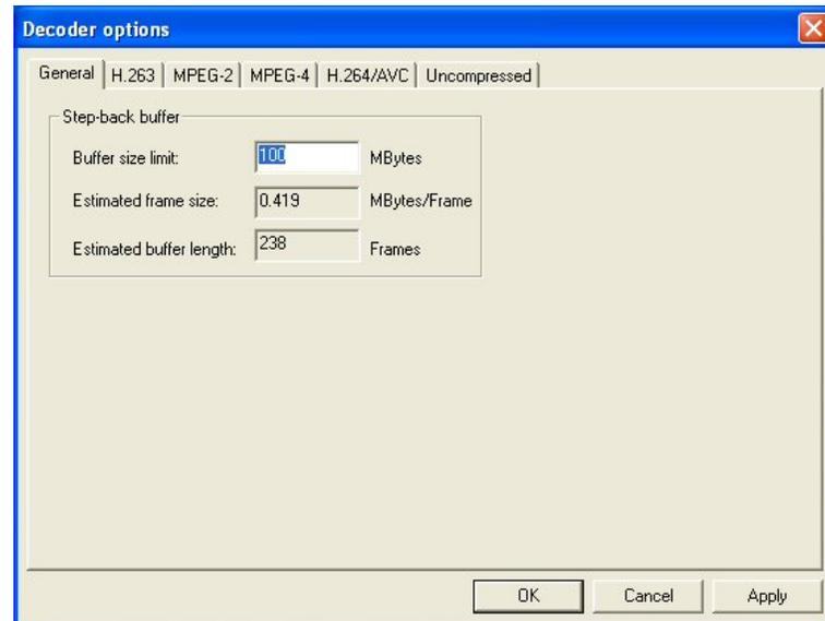
**Step-back buffer.** This buffer is used to hold the video and associated data, to make video play (forwards and backwards) occur without delay.
