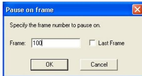
The last frame can be selected by using the Last Frame box. When this is done, the video pauses on the last frame. The previously entered frame number (if there is one) is still stored, and can be enabled again by clearing the Last Frame check box:
