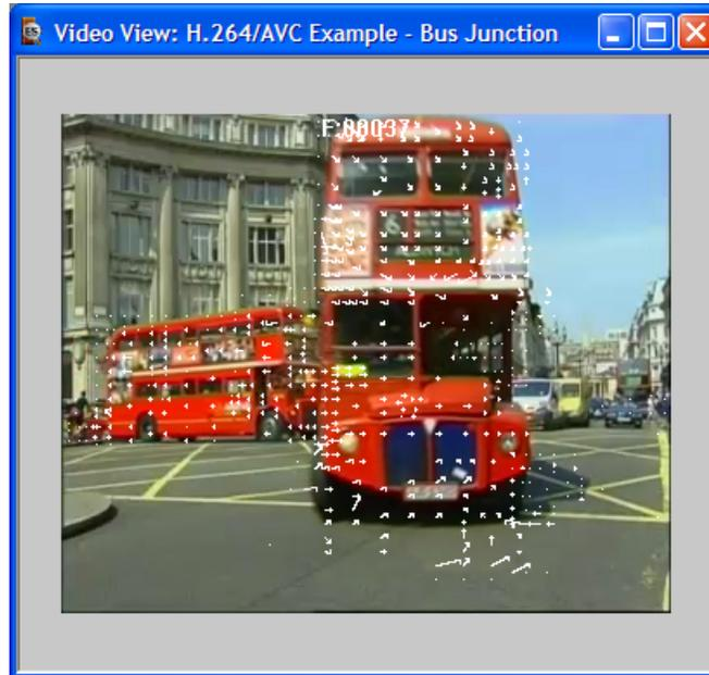
The motion vectors used in relevant video frames can be displayed on the frame currently being viewed. They are switched on and off by doing one of the following:
