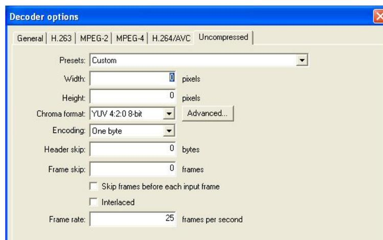
**Presets (Width and Height).** If there are numbers in the filename that could indicate the frame size, the MTS4CC will attempt to read these and offer these in the Width and Height fields shown in the previous screenshot. The correct values can be entered or selected using the drop-down list:
