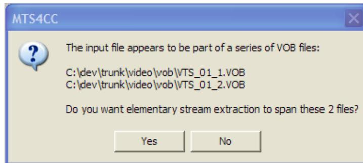
Clicking Yes means that the MTS4CC will extract the video Elementary Stream from all the VOBs indicated; clicking No means that the MTS4CC will only select the Elementary Stream from the VOB selected in the File open dialog box.
