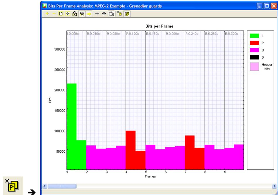
The bits per frame can be measured by selecting the toolbar measurement tool, placing the crosshair cursor over the point to be measured, and reading the result from the left side of the status bar.
