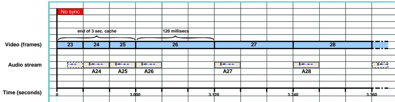
The preceding illustration shows an unsuccessful attempt to synchronize audio and video: the cached data plays in sync, thereafter, limited processor power causes the audio to fragment (usually more unevenly than suggested in the illustration) because it attempts to keep pace with the video by means of timestamps.
