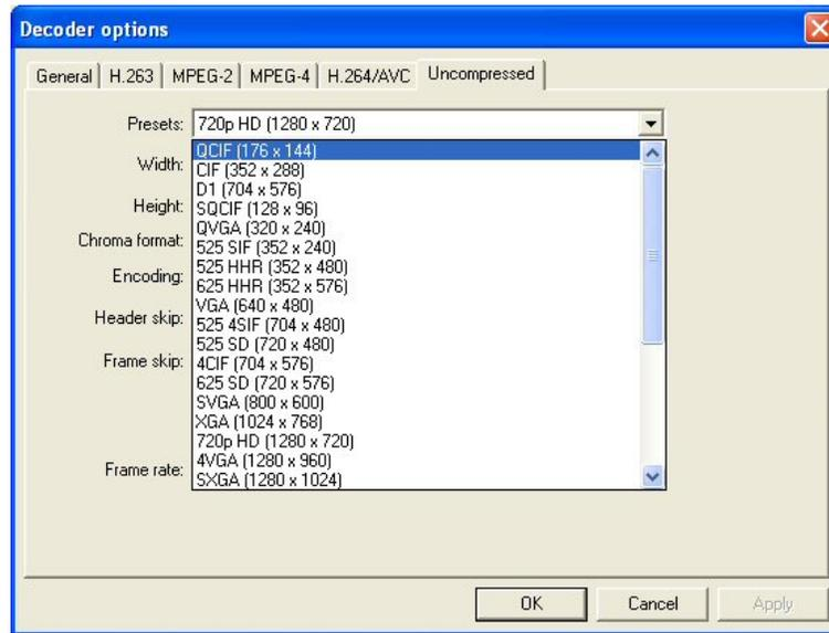
**Chroma format.** This control specifies the color model and format for the uncompressed video data. The combo provides several common combinations, including 8-bit YUV 4:2:0, 8-bit YUV 4:2:2, 8-bit YUV 4:4:4, 8-bit RGB and 8-bit grayscale. Select an entry from the list to use one of these common formats. Other formats can be specified by choosing the Custom entry in the list - this will open the Image format dialog.
