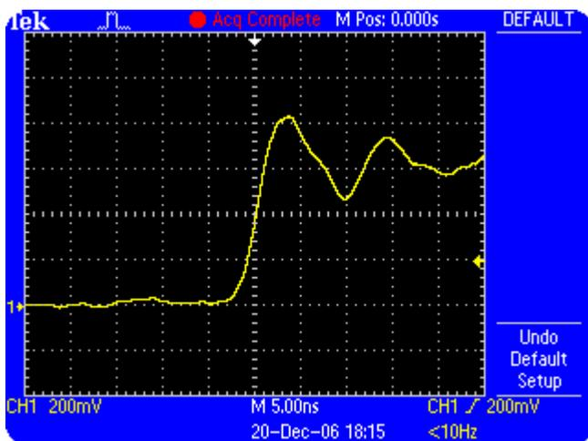
**Figure 5.7: Step response waveform with a ground lead**
