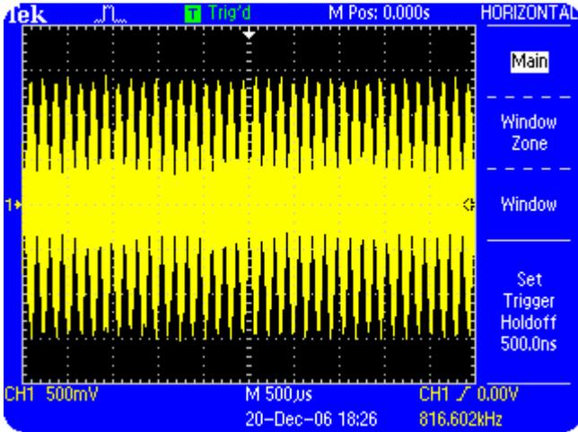
**Figure 5.11: Complex AM signal without holdoff**
