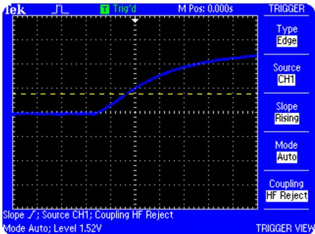
**Figure 5.3: Triggering waveform with HF Reject coupling**
