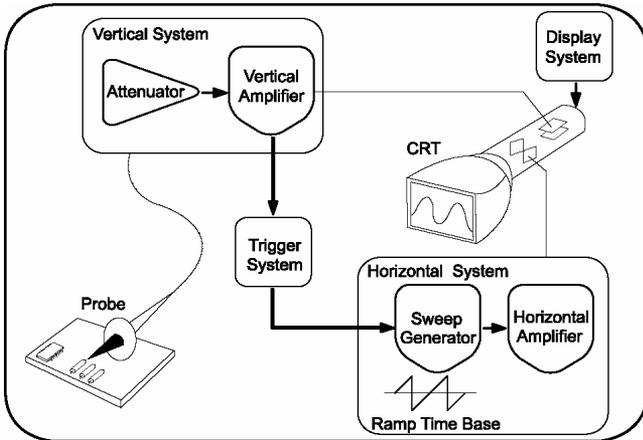
**Figure 1.3: Block diagram of an analog oscilloscope**
