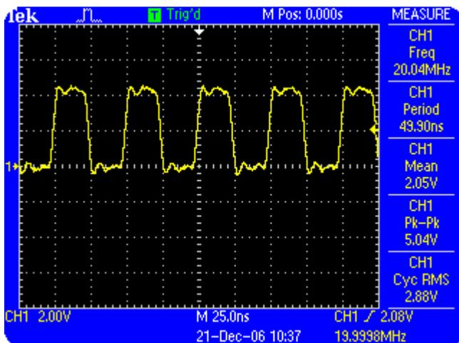
**Figure 6.13a: Square waveform with five automatic measurements**
