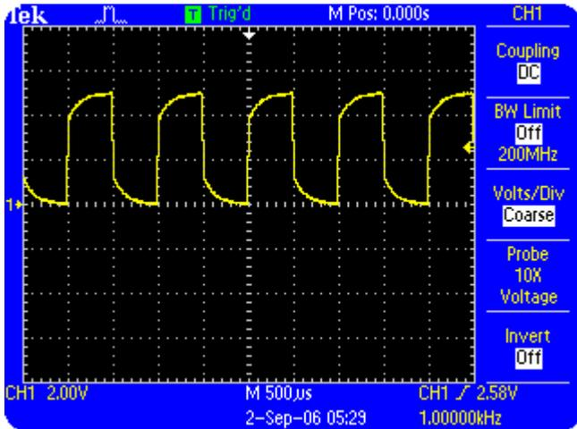
**Figure 2.6: Probe undercompensated**
