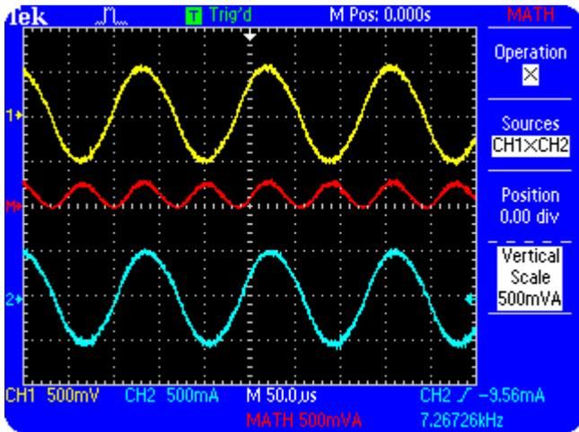
**Figure 3.6: Display of CH1xCH2**
