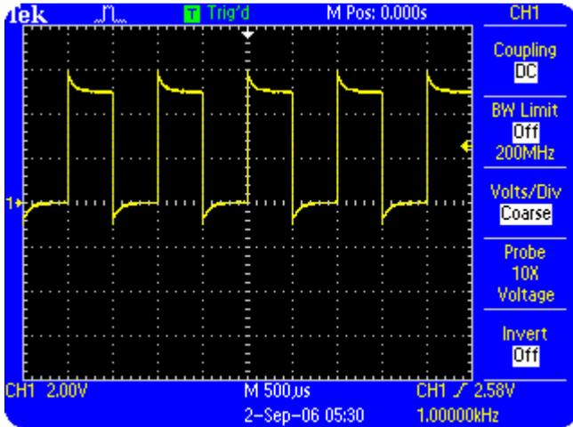
**Figure 2.7: Probe overcompensated**
