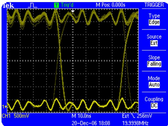
**Figure 5.4:** Eye Diagram display of pseudo random signal triggered by external clock signal
