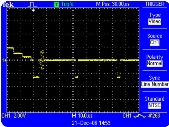
**Figure 2.14c: Triggering on video lines**
