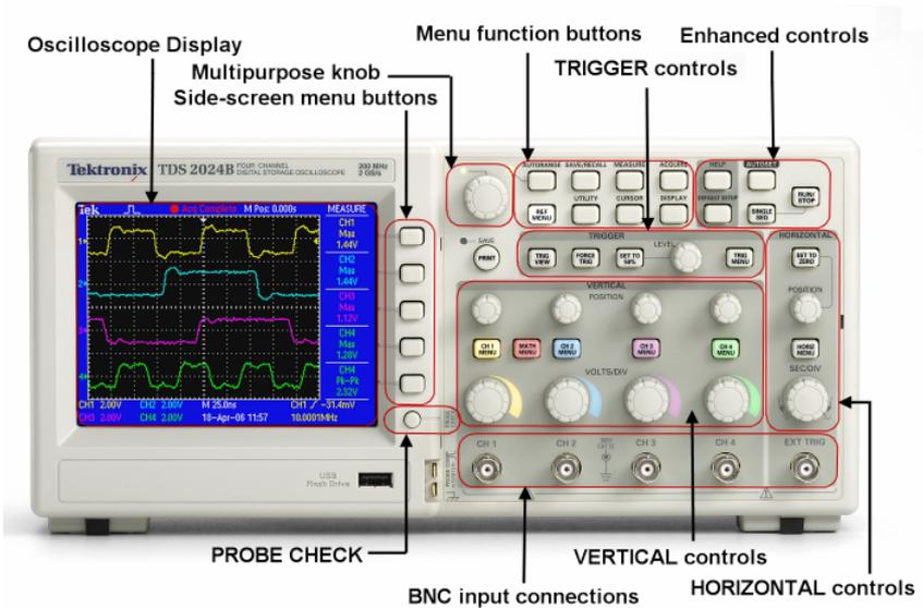
**Figure 2.2: The TDS2024B digital storage oscilloscope**
