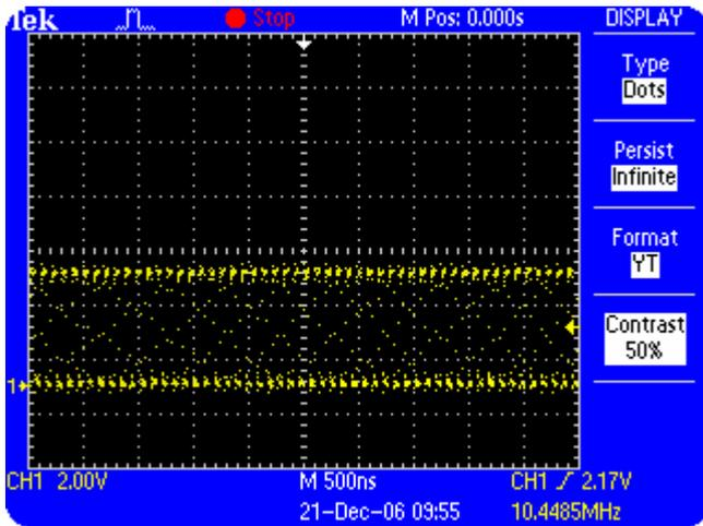
*Figure 6.7: A noisy signal with the final waveform acquisition dots displayed*
