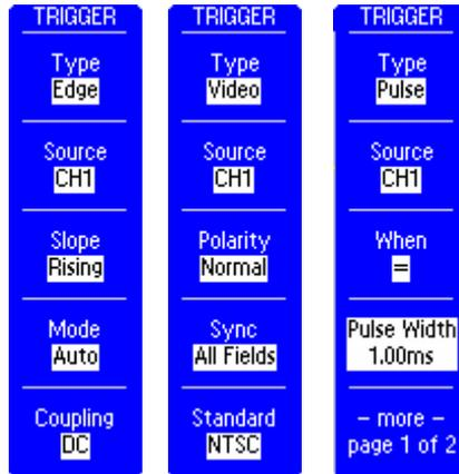
*Figure 2.14: Menu-based options for the TRIGGER controls*
