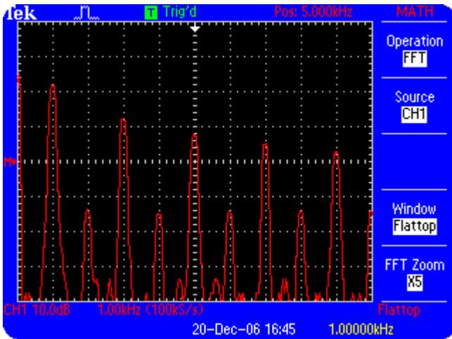
*Figure 3.7: FFT display of the calibrator signal*
