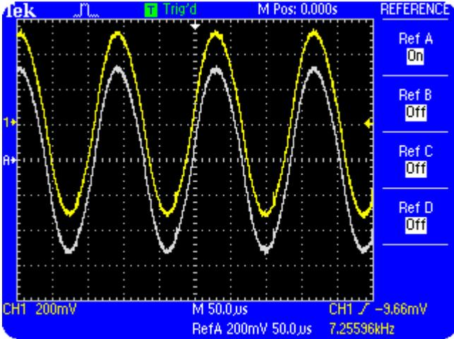
**Figure 6.15: Saved and updating waveforms displayed**
