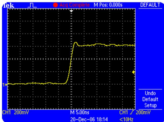
**Figure 5.8: Step response waveform without a ground lead**
