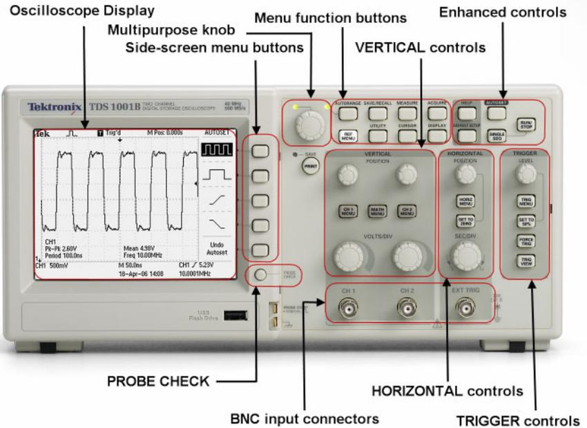
**Figure 2.1: The TDS1001B digital storage oscilloscope**
