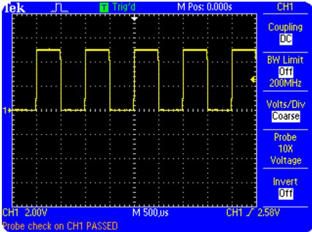
**Figure 2.5: CH1 probe compensation signal**
