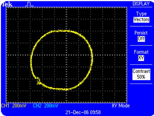
**Figure 6.8: XY Display of two sine waves with 90° phase shift**
