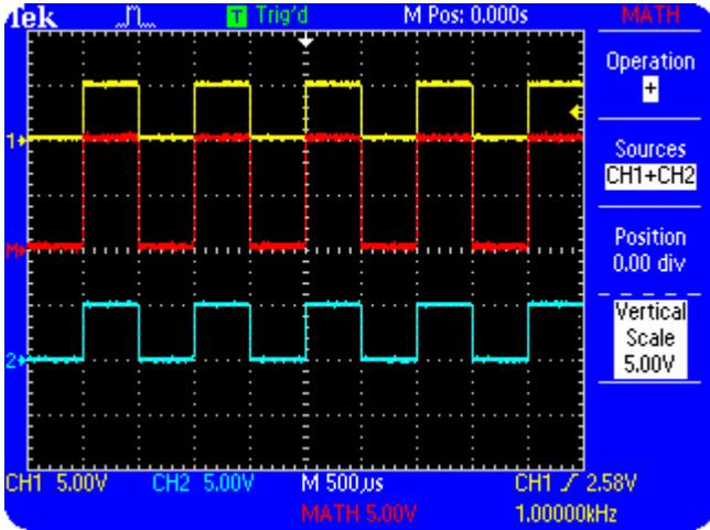
*Figure 3.4: Display of CH1+CH2*
