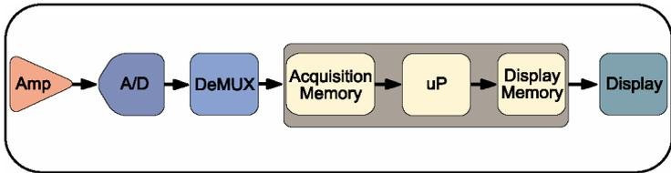
**Figure 1.5: Block diagram of a DSO**
