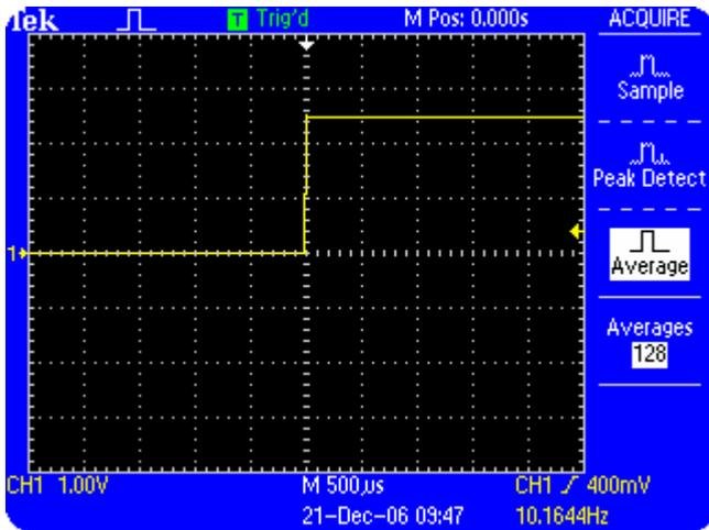
*Figure 6.4: A noisy variable amplitude signal acquired with the Average acquisition mode*
