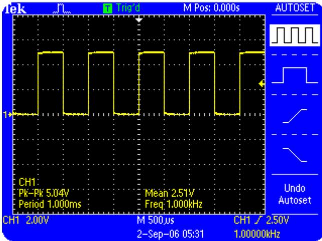
*Figure 4.2: TDS2000B horizontal setup*
