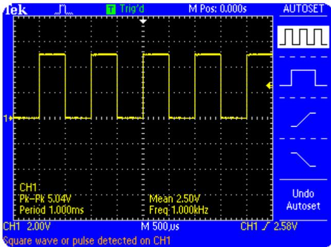
**Figure 2.3: Square wave of 5 volts peak-to-peak at 1 kHz**
