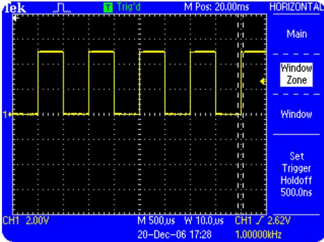
*Figure 4.4: Position delayed and Window Zone*
