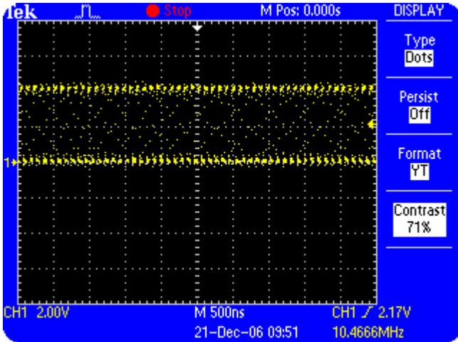
**Figure 6.5: Waveform displayed in dots**
