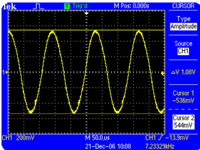
**Figure 6.9: Volts/amplitude measurement for a 5 kHz sine wave**
