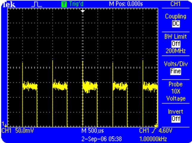
**Figure 3.3: Vertical display, with 100 divisions of offset**
