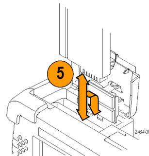
You can add a second battery to increase the operating time. Replace a battery with the specified type only. To purchase a battery, contact your Tektronix Service Center for the correct part number.
