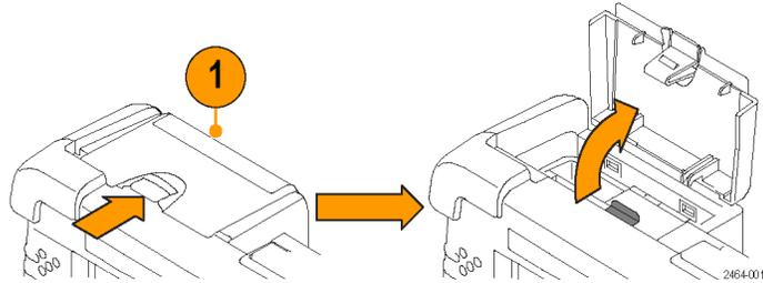
2. Push the metal battery retainer tab down and towards the back of the instrument.
