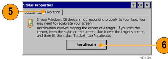
7. Follow the target screen instructions. When the position target disappears, touch anywhere on the screen to return to the Calibration tab.
