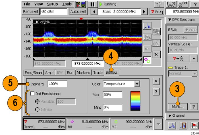
7. Use the **Color** field to set the color scheme used for the Bitmap trace.
