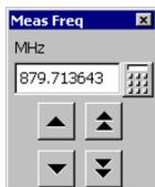
The Increment control lets you use buttons to increase or decrease the value of the field in small or large steps. The single arrow buttons make small changes. The double arrow buttons make larger changes.
