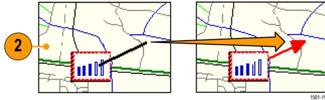
3. To change the arrow direction, draw a new line. iMap replaces the existing arrow with the new direction arrow.
