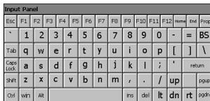
WindowsCE provides an Input Panel (virtual keyboard) that you can use to enter text such as file names. In most cases, when the instrument opens a dialog box that includes fields for text entry, the Input Panel also opens. When you close the dialog box, the Input Panel also closes.
