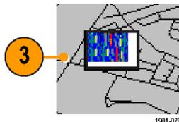
4. You can select a different measurement button, and then tap the map to add a new measurement to the map. Multiple measurement icons at the same location stack on top of each other.
