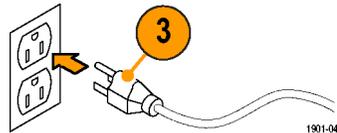
4. Charge the batteries before using the instrument on battery power for the first time. (See page 7, *Charging the Batteries*.)
