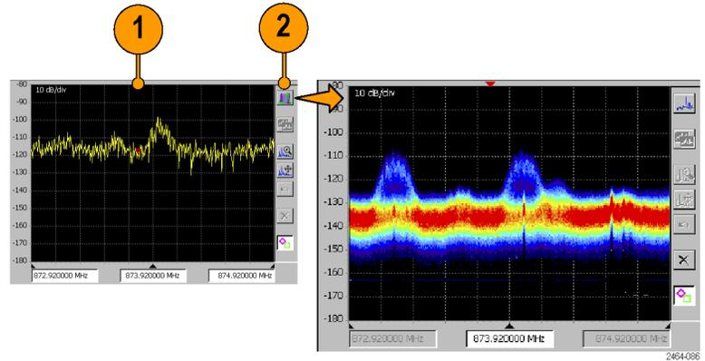
3. Tap the **More** button in the DPX Spectrum drawer to display the DPX spectrum parameter tabs.
