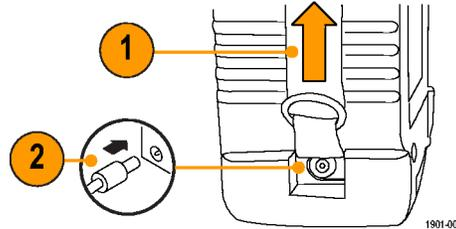
3. Connect the AC adapter to a properly-grounded AC power source using the provided power cord.
