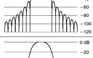
A plot showing the magnitude response of a Sine to the 4th window. The main lobe is a smooth curve peaking at 0 dB. The side lobes are smaller than in the Parzen window. The y-axis is labeled from 0 dB to -120 dB in increments of 20 dB.                    | 1.85      | -47 dB    | 1.944444 |
