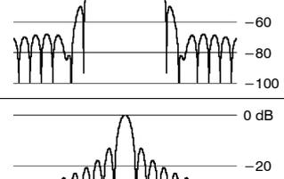
A plot showing the magnitude response of a Flat Top window. The main lobe is a smooth curve peaking at 0 dB. The side lobes are smaller than in the Parzen window. The y-axis is labeled from 0 dB to -100 dB in increments of 20 dB.                           | 3.182     | -51 dB    | 3.196927 |
