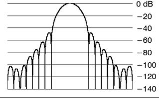
A plot showing the magnitude response of a Rosenfield window. The main lobe is a smooth curve peaking at 0 dB. The side lobes are significantly smaller than in the Parzen window. The y-axis is labeled from 0 dB to -140 dB in increments of 20 dB.             | 1.814     | -48 dB    | 1.90989  |
