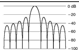
A plot showing the magnitude response of a Parzen window. The main lobe is a smooth curve peaking at 0 dB. The side lobes are smaller and more numerous than in other windows. The y-axis is labeled from 0 dB to -100 dB in increments of 20 dB.                 | 1.27      | -27 dB    | 1.330747 |
