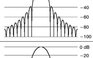
A plot showing the magnitude response of a Sine Cubed window. The main lobe is a smooth curve peaking at 0 dB. The side lobes are smaller than in the Parzen window. The y-axis is labeled from 0 dB to -100 dB in increments of 20 dB.                         | 1.654     | -39 dB    | 1.734891 |
