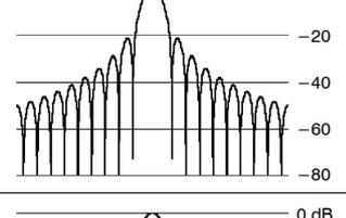
A plot showing the magnitude response of a Welch window. The main lobe is a smooth curve peaking at 0 dB. The side lobes are smaller than in the Parzen window. The y-axis is labeled from 0 dB to -80 dB in increments of 20 dB.                                 | 1.15      | -21 dB    | 1.197677 |
