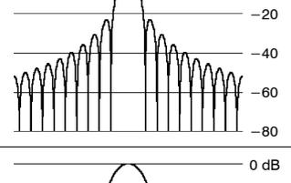
A plot showing the magnitude response of a Sine Lobe window. The main lobe is a smooth curve peaking at 0 dB. The side lobes are smaller than in the Parzen window. The y-axis is labeled from 0 dB to -80 dB in increments of 20 dB.                           | 1.186     | -23 dB    | 1.233702 |
