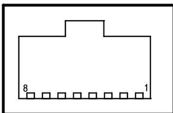
**Figure 1-1: Ethernet pinout**
