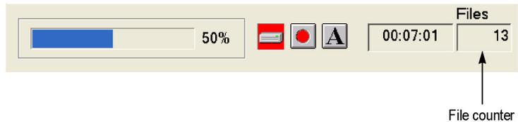
When the specified number of files are created or you press the front-panel Stop button, stream capture stops.
