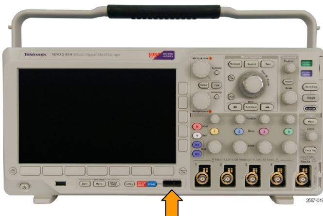
Figure 3-5: Digital channel input (MSO only)
