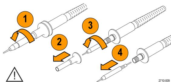
Securely tighten the insulator and new tip before using the probe. 2710-009
