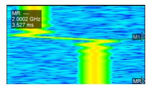
11. Use the mouse to move the MR marker in the Spectrogram display to a point of interest. As you move the marker up and down, look at the corresponding changes in the marker in the Spectrum display. The Time-Frequency Analysis application preset configured the Spectrum display to show the selected spectrogram line.
