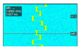
10. Right click the mouse and select Zoom from the resulting menu. Pull the mouse vertically and horizontally to zoom in on one or two hops of the spectrogram signal.
