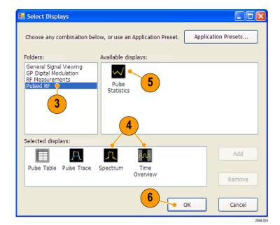
When Trend is the selected plot, the Pulse Statistics display plots the results of the selected measurement for every measured pulse.
