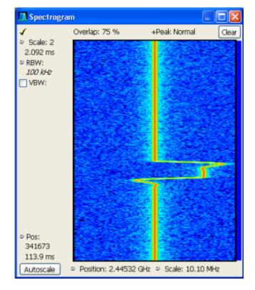
The Spectrogram display shows both time and frequency domains in a single display. The vertical axis is time, with newer data at the bottom. The horizontal axis is frequency, covering the same span as the Spectrum display.
