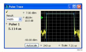
2. Click the Pulse control in the Pulse Trace display and enter a different pulse number.
