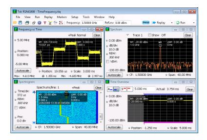
The *Frequency vs Time* display shows the deviation from the center frequency value on the vertical axis and time on the horizontal axis.
