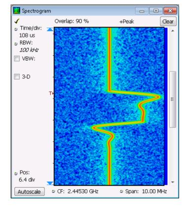
The Spectrogram display shows both time and frequency domains in a single display. The vertical axis is time, with newer data at the bottom. The horizontal axis is frequency, covering the same span as the Spectrum display.
