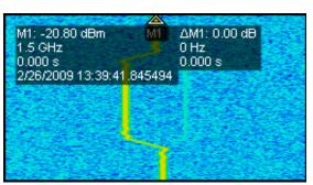
The *Time Overview* display shows log power on the vertical axis and time on the horizontal axis.
