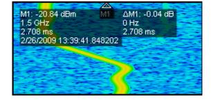
11. Use the mouse to move the MR marker in the Spectrogram display to a point of interest. As you move the marker up and down, look at the corresponding changes in the marker in the Spectrum display. The Time-Frequency Analysis application preset configured the Spectrum display to show the selected spectrogram line.
