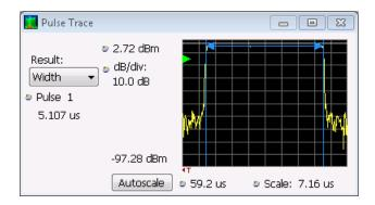
2. Click the Pulse control in the Pulse Trace display and enter a different pulse number.
