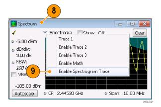
The Spectrogram trace in the Spectrum display corresponds to the line selected in the Spectrogram display by the active marker.
