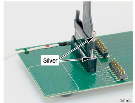
**Figure 5: P6750 Probe connection**
