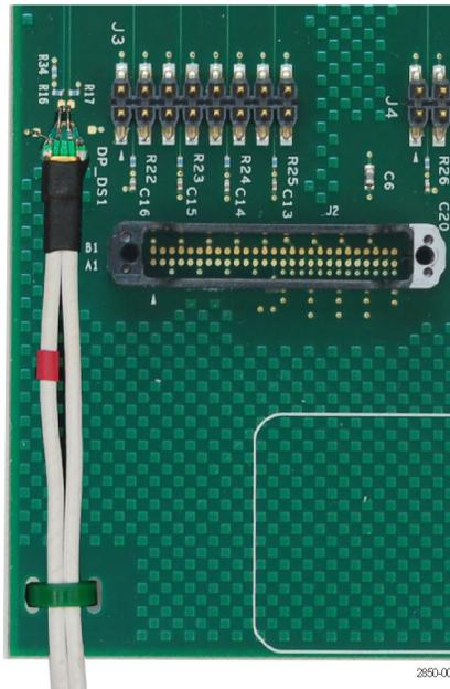
**Figure 2: P75TLRST solder tip connections**
