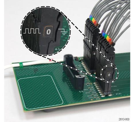
**Figure 3: Single-ended probe connections**
