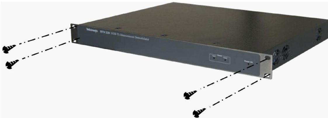
Figure 4: Securing the instrument in an equipment rack
