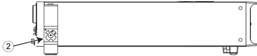
Figure 9: Remove mounting ears
