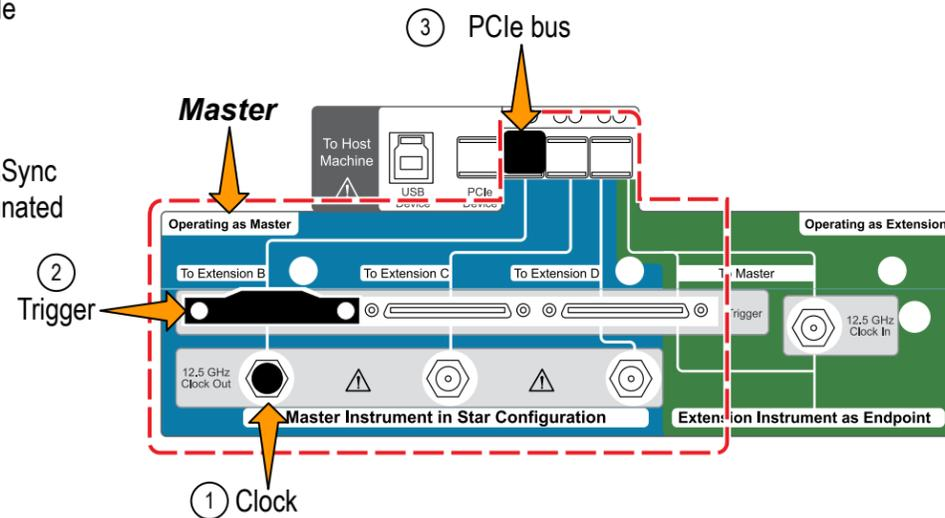
Connecting UltraSync bus cable bundles on Extension
