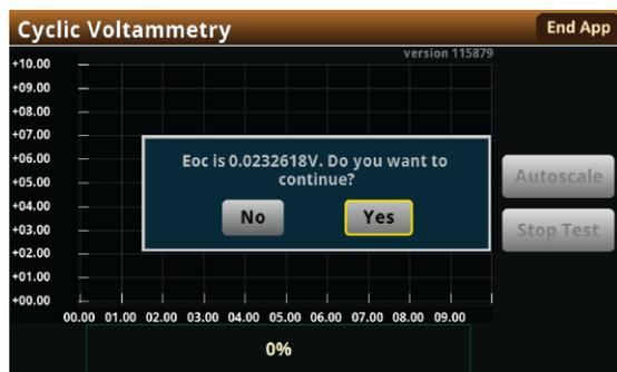
If this value is acceptable, then select **Yes** to start the scan. If you select **No**, the test will stop. The measured Eoc value is saved in the `eocBuffer` internal buffer of the instrument.
