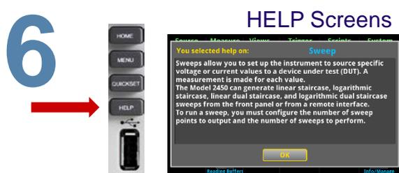
On the front panel, press the **HELP** key. The SMU has a context-sensitive help system to speed up your learning curve. When an icon or touchscreen button has focus (icon or button is highlighted with a yellow box), that feature or function has context-sensitive help. If there is no specific focus when you press the **HELP** key, overview information for the screen you are viewing displays.
