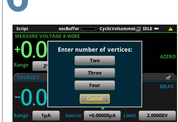
After the open circuit voltage is measured, the parameters of the potential sweep must be defined: Number of vertices, voltage magnitude, and reference voltage.
