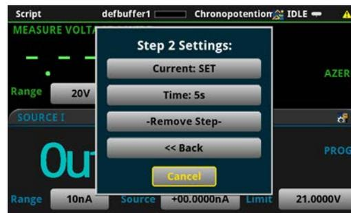
Add a second step to discharge the battery
