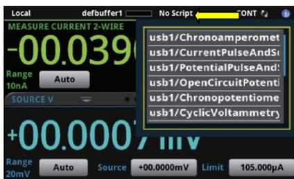
Your Model 2450-EC or 2460-EC demo system came with preloaded electrochemistry test scripts. The demo system also came with a flash drive that contains all of the test scripts and documentation for your reference.
