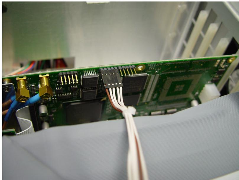
**Figure 10: Interface cable connected to the hardware upgrade module**
