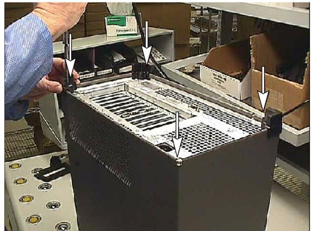
Figure 12: Removing the handle and feet from the cabinet
