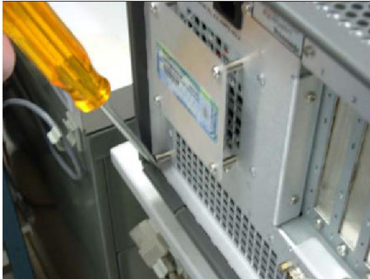
**Figure 13: Prying the cabinet loose from the chassis**
