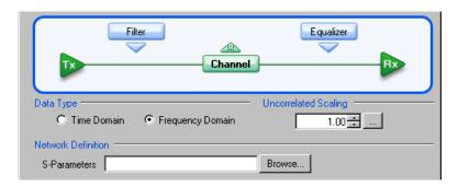
The S-parameters file can contain data for 1-port, 2-port, or 4-port devices. Once a file is selected, the application reads its contents and generates the appropriate dialog for you to select the particular S-parameter in the file to use.
