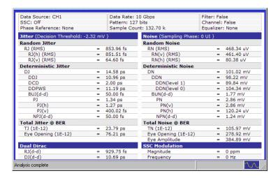
You can easily switch between summary and detailed numeric displays with the use of the numeric results button and the plot window buttons
