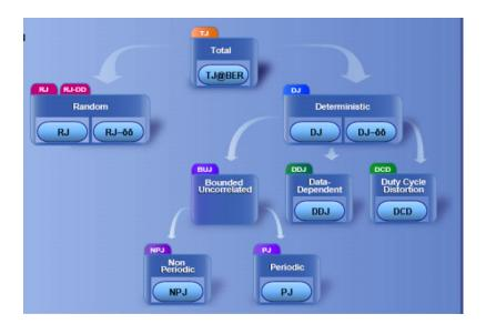
Bit error rates (BER) of a serial data stream are impacted by both jitter and noise. An accurate decomposition of jitter and noise in the sources of impairments is critical to correctly estimate the signal path behavior at larger BER. The jitter and noise maps are critical to help debugging the devices under test.
