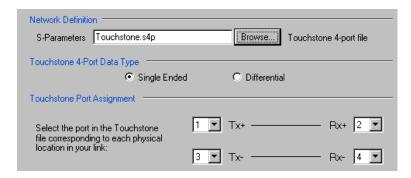
If the data is mixed mode, you must select the data layout in the file. The most common layout is DC12 and is the default selection. The application always uses the  $S_{dd21}$  parameter for computing the transmitted waveform no matter which mapping is selected.
