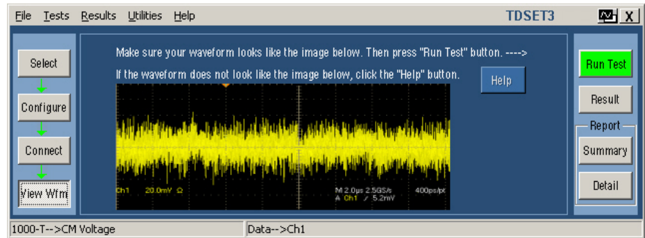
Figure 11-13: 1000BASE-T View Waveform for CM Voltage
