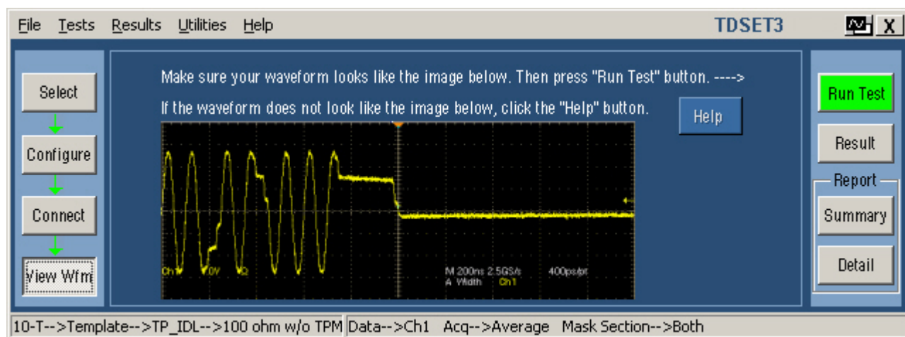
Figure 13-4: 10BASE-T View Waveform for TP_IDL without TPM
