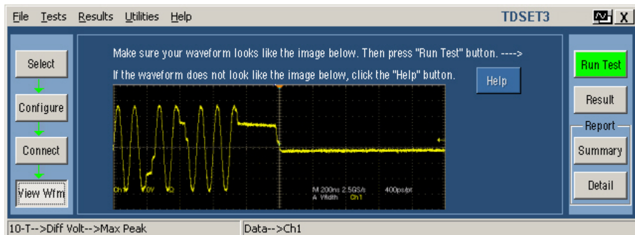
Figure 13-7: 10BASE-T View Waveform for Differential Voltage
