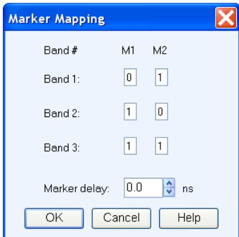
You can set the following options for markers M1 and M2. The marker pattern generated, based on the following settings, can be used for triggering an external device.
