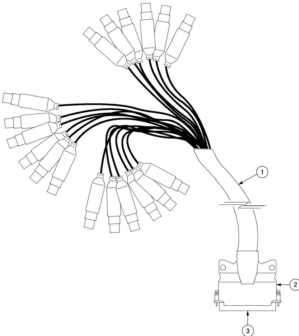
**Figure 5- 4: Analog audio breakout cable assembly**
