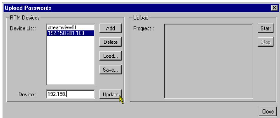
The **RTM Devices** pane displays the addresses of the DTV monitors that the Passwords file will be uploaded to when **Start** is selected.
