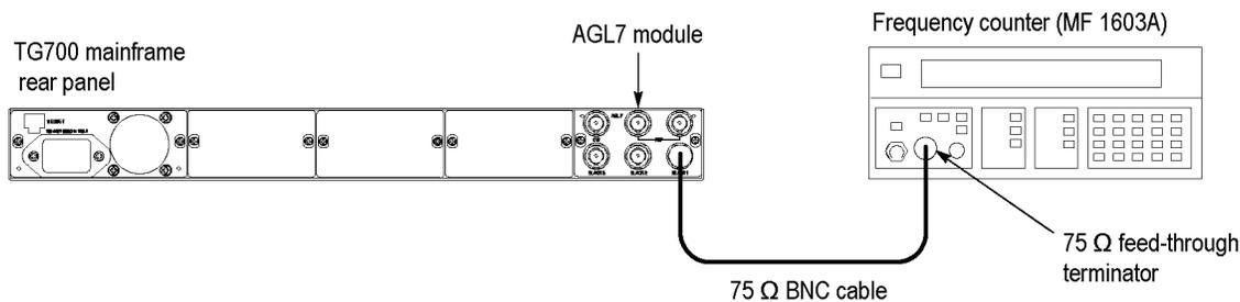
**Figure 2: Equipment connection for verifying subcarrier frequency**
