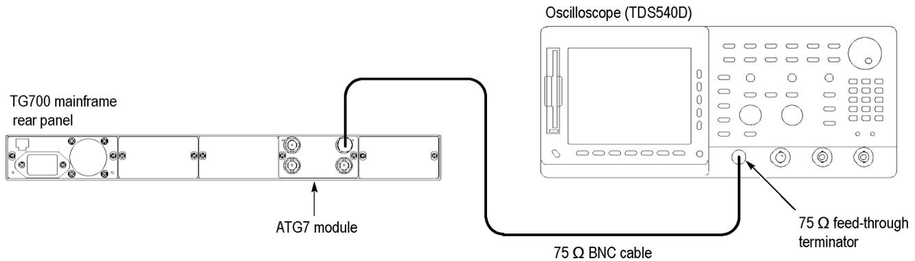
**Figure 12: Equipment connection for verifying pulse amplitude**
