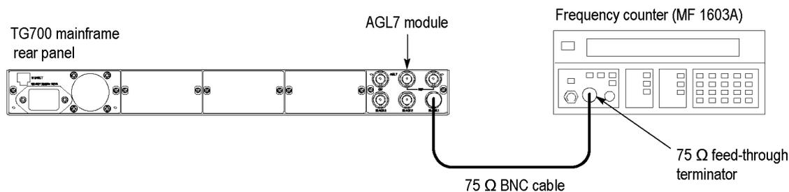
**Figure 9: Equipment connection for verifying subcarrier frequency**
