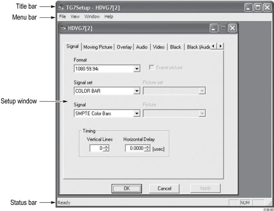
Figure 2: TG7 Setup application window
