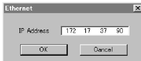
**Figure 1: Ethernet dialog box for TG7 Setup**
