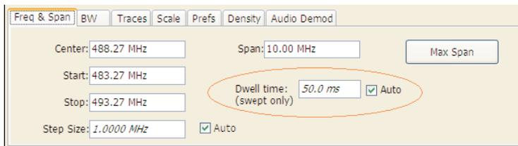
Figure 15. During swept DPX operation, the Dwell time control adjusts the observation time of each frequency segment used to construct the composite DPX spectrum display.
