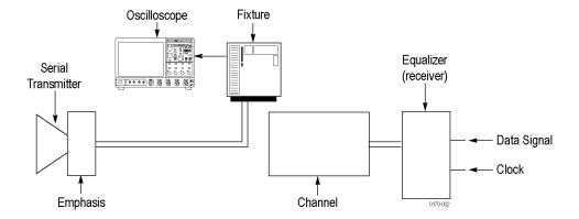
The Rx button configures the software to match your system as shown in the following figure. The oscilloscope is connected to the Fixture as shown. The Fixture, when enabled, provides access to the receiver side of the transmission Channel. By de-embedding the Fixture, you effectively move the oscilloscope connection right to output of the Channel. This setup allows you to de-embed the transmission channel and see the quality of the transmitter signal at TpB.
