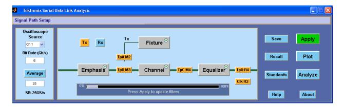
The circuit blocks use either Tektronix supplied S-parameter files or an S-parameter or FIR filter file supplied by you. Once you have selected appropriate filters for all enabled circuit blocks, you click Apply and the software generates FIR filters for all enabled blocks. You can review the response of the filters by clicking the Plots button. This is a good way to verify that you have loaded the right filters and set appropriate cutoff frequencies with the Bandwidth Limit function.
