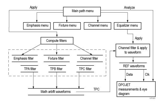
Test point filters for TpA, TpB, and TpC are created by convolving them with combinations of the circuit block filters as shown in the table.
