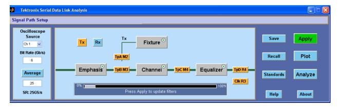
The Fixture and Circuit blocks embed or de-embed their effects on the source signal. You can configure any block by clicking on it. The test points (TpA, TpB, and TpC) show the effects of the blocks on the source signal.
