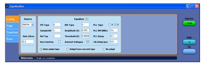
The bit rate you enter must be accurate to recover the data and clock signals. The software performs clock recovery by emulating a phase locked loop (PLL) circuit. Use the data rate defined for the serial standard you are testing. If you are testing a new serial line, you may need to measure the bit rate near the Transmitter.
