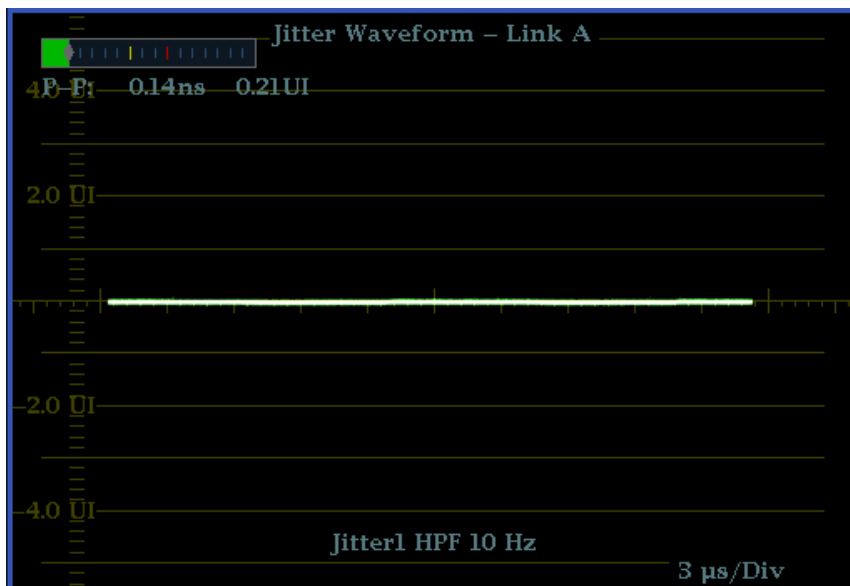
Figure 36: The Jitter display parameters as shown in a single tile when the instrument is in 4-tile mode
