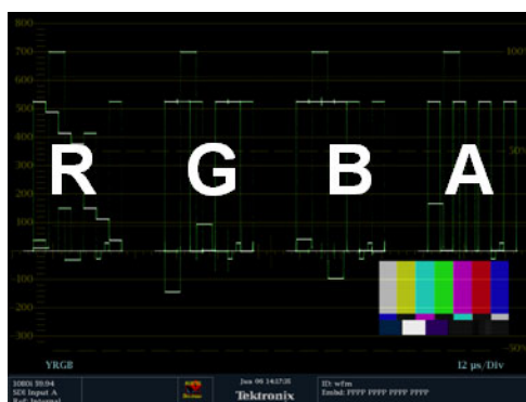
Figure 14: Dual Link information placement in waveform display
