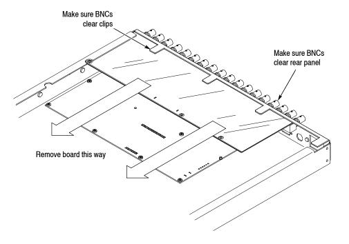
**e.** Keep the spacer plate that goes between the BNCs and the rear panel.
