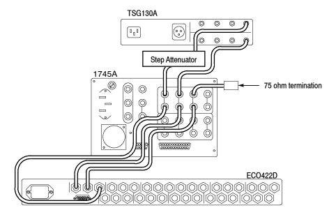
Figure 1-6: Setup for adjusting R265 (the user level for SX-7)
