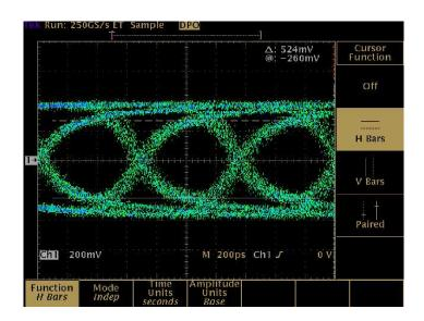
Figure 2-1: Typical eye-pattern of 20 m of Belden 1694A cable
