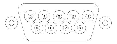
Figure 1-4: Remote connector pins
