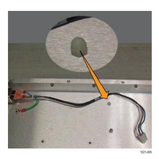
**4.** Install the remote connector on the rear panel as shown in the following figure.
