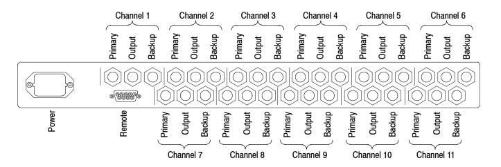
Figure 1-3: Rear panel of the ECO422D
