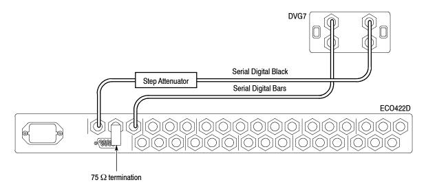
Figure 4-2: Setup to check the component serial digital video levels
