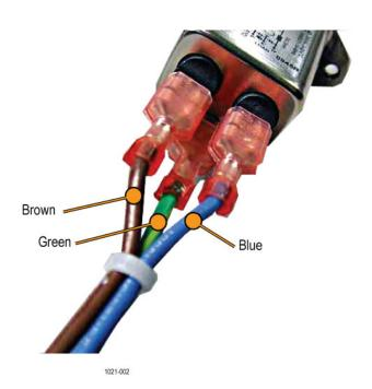
**b.** With the ground lead (green wire) toward the bottom of the chassis, insert the line filter through the back of the rear panel as shown in the following figure.
