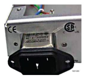
**c.** Place the connector plug you removed from the old chassis on the line filter, and then attach the plug to the chassis as shown in the following figure.
