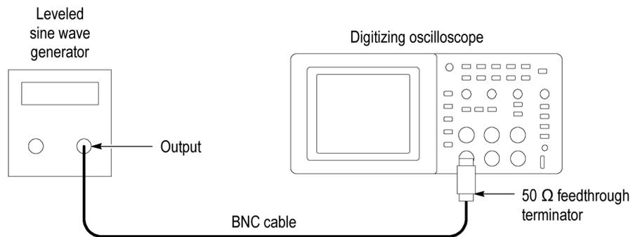
3. Set the oscilloscope **Vertical Scale** (volts/division) to **500 mV/div**.
