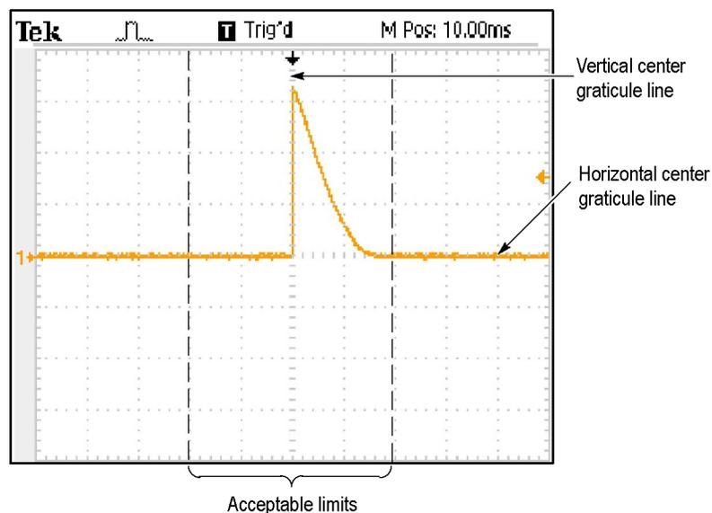
**NOTE.** One division of displacement from graticule center corresponds to a 25 ppm time base error.
