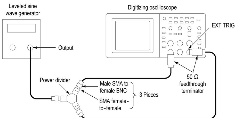
3. Set the oscilloscope **Vertical Scale** (volts/division) to **100 mV/div**.
