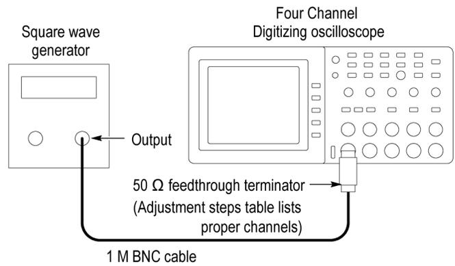
**Figure 5-1: Adjustment setups**
