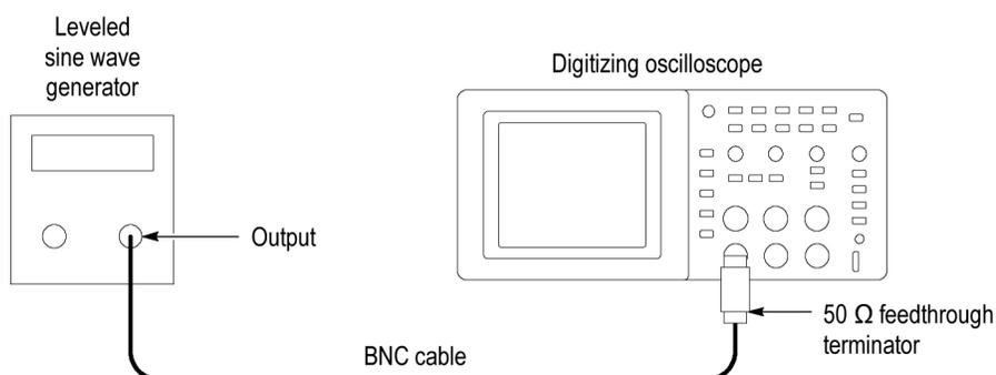
3. Set the oscilloscope **Vertical Scale** (volts/division) to **500 mV/div**.
