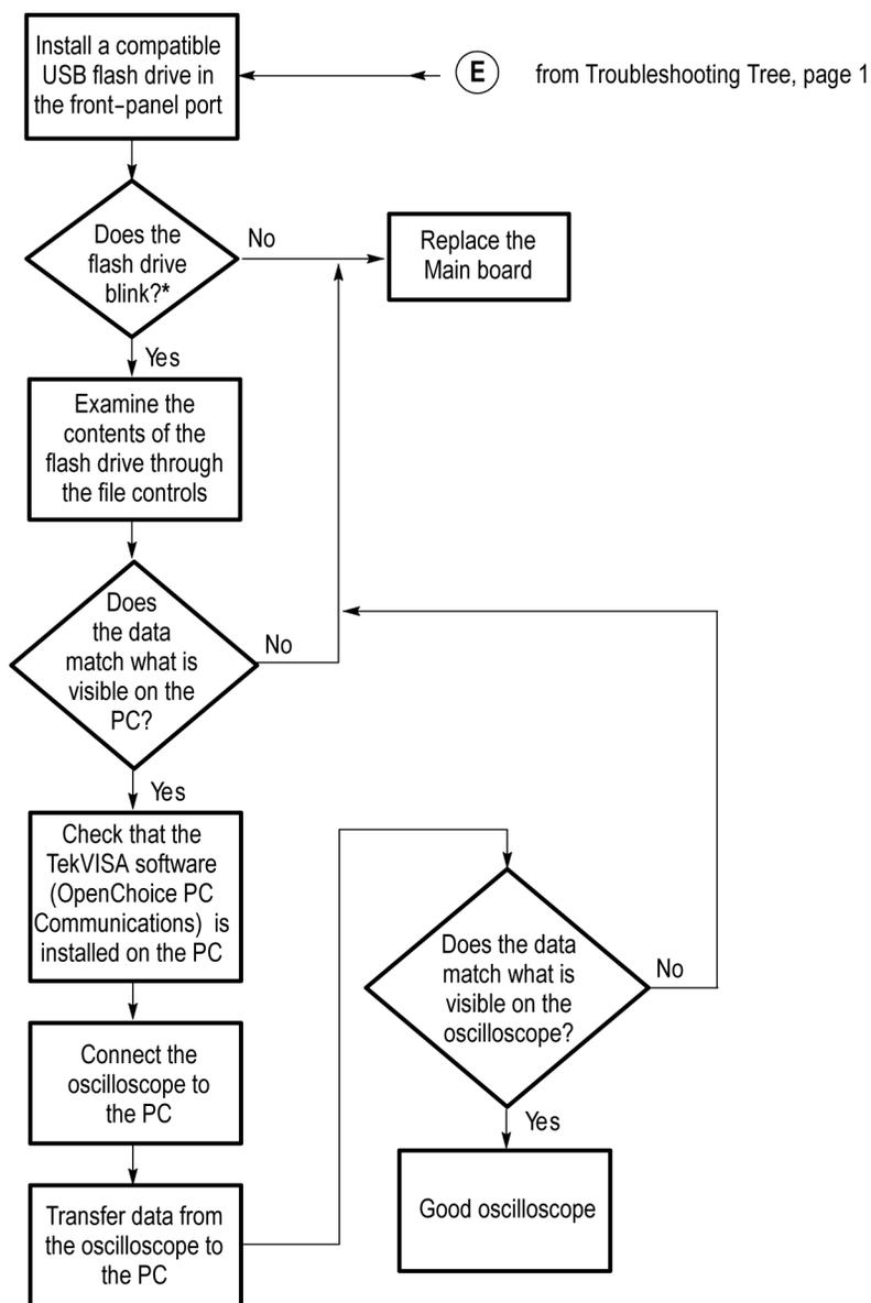
\* The oscilloscope displays a clock symbol when the flash drive is active, and a hint line when a save or recall operation is complete.
