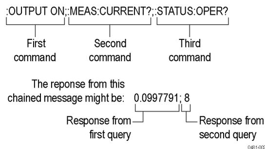
**Figure 2-4: Example of chaining commands and queries**
