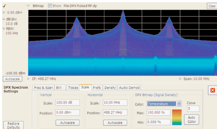
Figure 8. DPX spectrum bitmap with default color scale settings.
