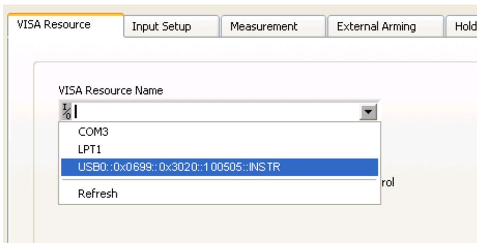
For network-connected instruments, the VISA Resource list shows the IP Address of instruments connected to the network, instead of instrument-generated identifier text. Select the IP address assigned to the instrument to which you want access. (See page 8, *Ethernet Cable*.)
