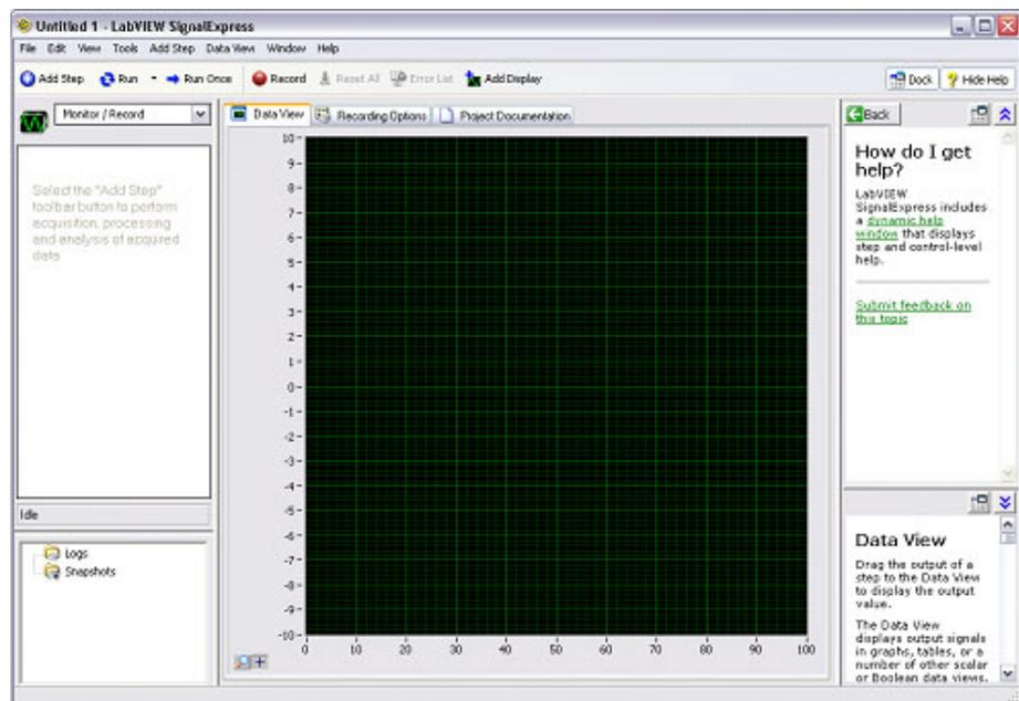
5. Add the Step that supports your instrument: click **Add Step > Tektronix > Acquire Signals** (for measurement instruments) or **Add Step > Tektronix > Generate Signals** (for signal source instruments) and select the Step that supports your instrument. SignalExpress loads the selected Step and displays the Visa Resource tab.
