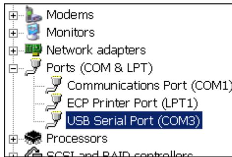
5. Record the instrument USB serial COM port number for use with the SignalExpress software.
