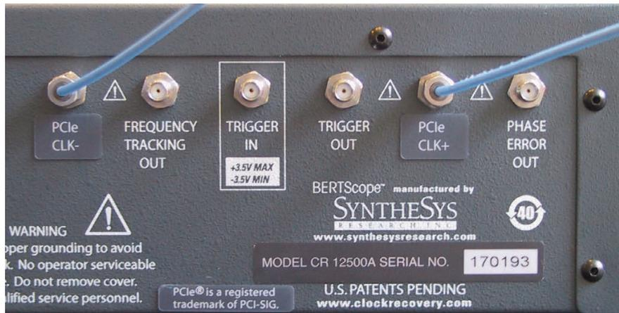
The PCIe CLK+ and PCIe CLK- connectors are located on the front panel of the model PLL-PCIE analyzer. The REF\_CLK input connector locations on the CBB are shown below.
