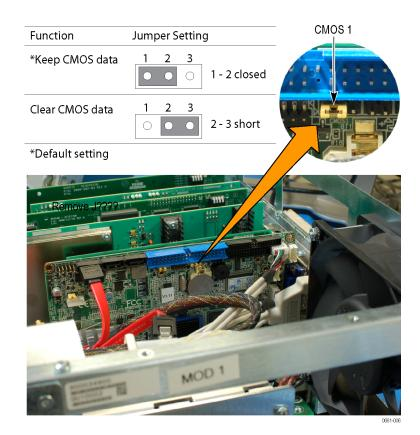
**4.** Move the jumper to the pin 2–3 position.
