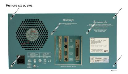
4. Slide the instrument chassis out from the enclosure and set it aside.
