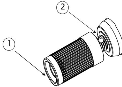
There are two locations on the binding post to connect the wire. See the picture above. You can use one of the methods below to connect the outputs from the front panel:
