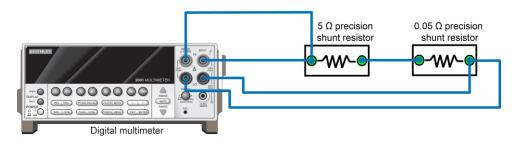
After connection, you can read the shunt value from the DMM ( $R_{total}$ ). Make sure the  $R_{total}$  is within the range of 5.05 ± 0.05  $\Omega$ . If it is not, adjust your shunts to guarantee the total shunt value is in the required range.
