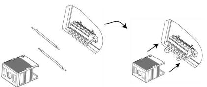
Use the following steps to short the output terminals and sense terminals:
