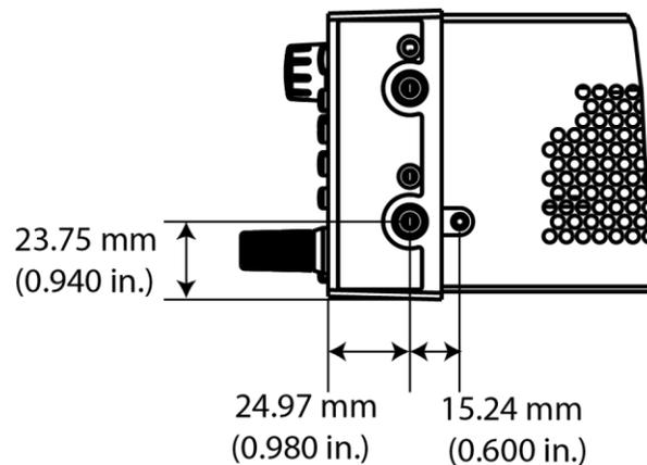
The following figures show the dimensions when the bumpers are installed.
