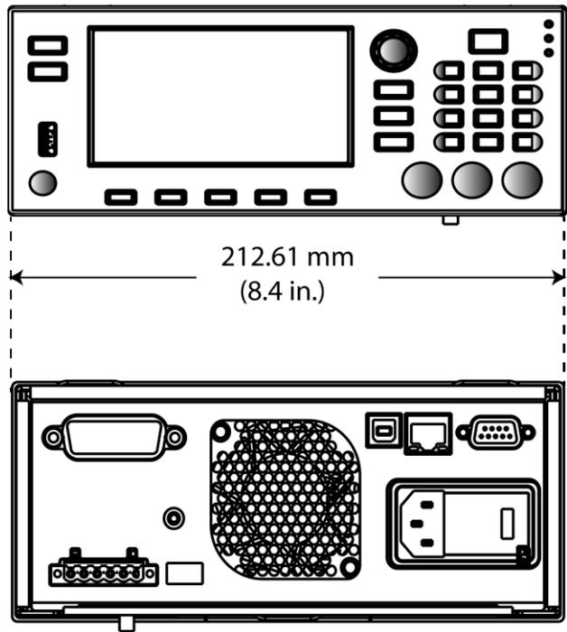
Figure 20: Series 2280 top and side dimensions with bumpers removed
