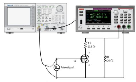
Figure 89: Fast current measurements setup
