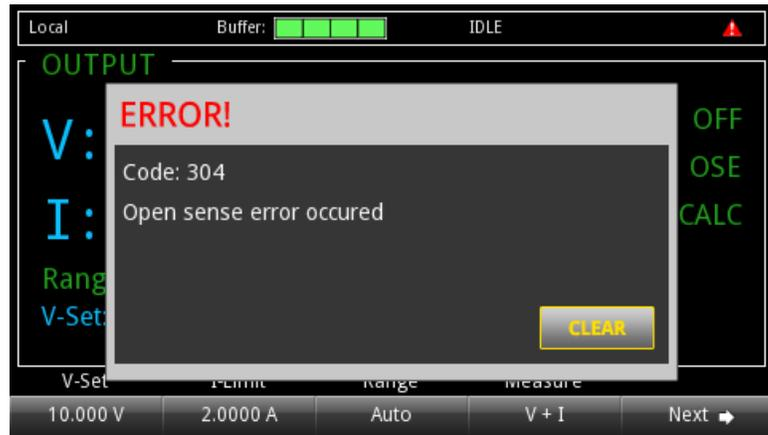
You can retrieve the error number and message through a remote interface by sending the `:SYSTEM:ERROR?` command.
