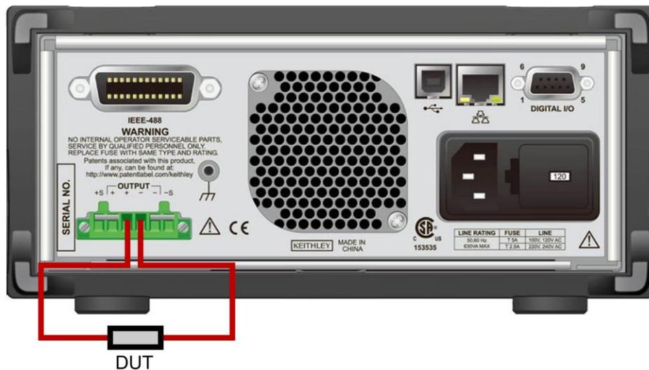
If you use a two-wire sense connection, you can use the offset function of Series 2280 to cancel out the wire resistance. For details, refer to [Relative offset](#) (on page 4-12).
