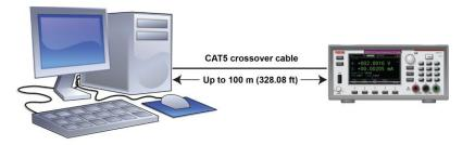
Figure 34: One-to-one connection with a crossover cable
