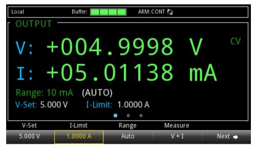
Figure 84: Voltage and current readback
