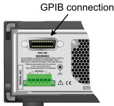
3. Connect any additional connectors from other instruments, as required for your application.
