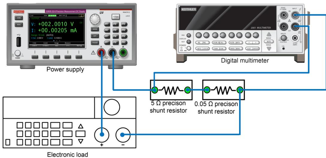
Figure 114: Measure the voltage across the 0.05 ohm shunt
