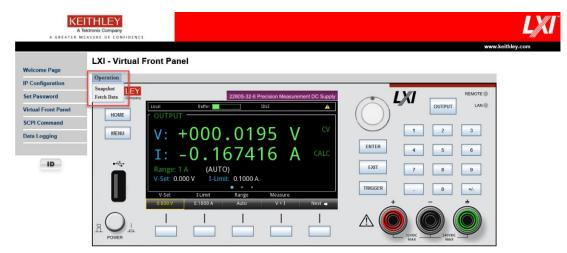
Figure 42: Series 2280 Virtual Front Panel
