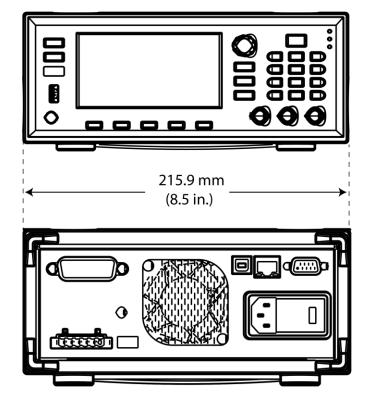
Figure 17: Series 2280 front and rear panel dimensions with bumpers
