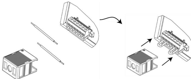
Use the following steps to short the output terminals and sense terminals:
