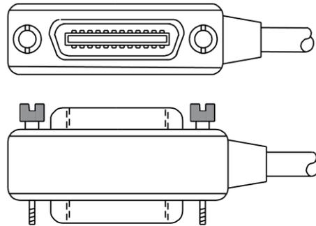
To allow many parallel connections to one instrument, stack the connectors. Each connector has two screws on it to ensure that connections remain secure. The figure below shows a typical connection diagram for a test system with multiple instruments.
