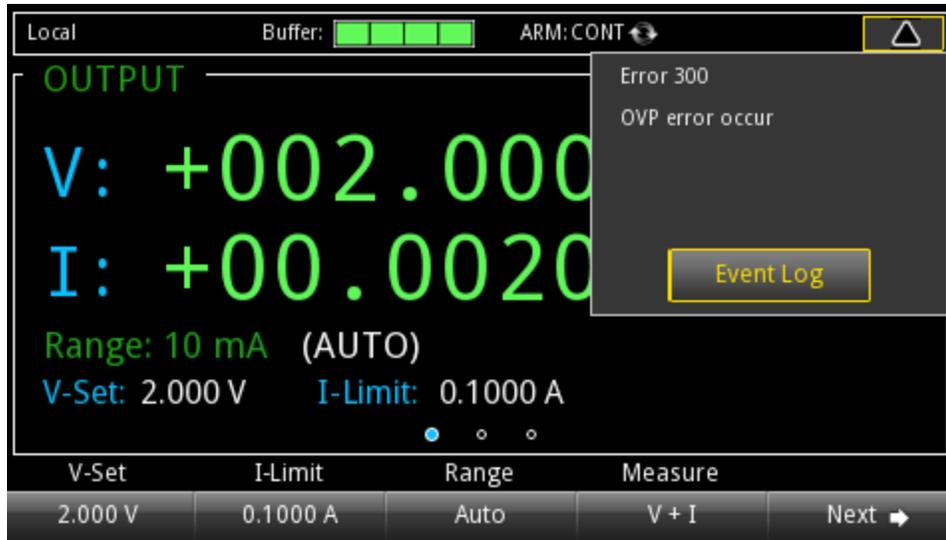
This indicator has a different appearance based on the type of event that has been logged.
