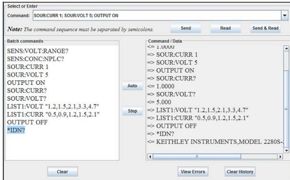
2. In the **Command** box, enter the SCPI command. You can enter a single command or batch commands, as shown in the figure.
