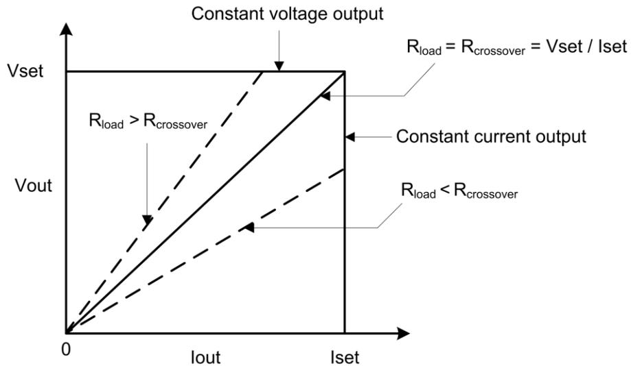
For example, if the resistive load is such that the power supply is operating in constant-voltage mode, the power supply provides a regulated output voltage. As the load increases, the output voltage remains constant until the preset current limit is reached. Then the crossover occurs.
