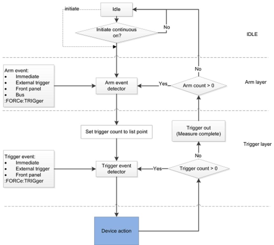
As shown in the previous figure, the device action can be any mode described in [List running time](#) (on page 3-44). The measurement time is set accordingly.
