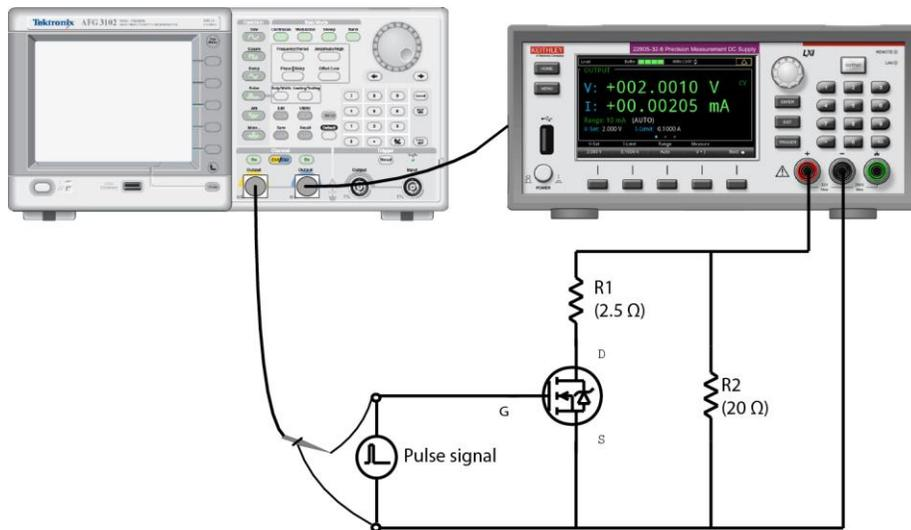
Connect the digital I/O pin 1 and pin 9 with the AFG output channel. For details on digital I/O, refer to [Digital I/O](#) (on page 3-19).
