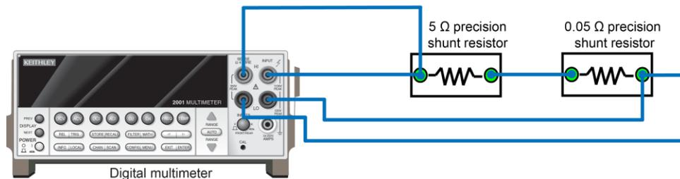
After connection, you can read the shunt value from the DMM ( $R_{total}$ ). Make sure the  $R_{total}$  is within the range of  $5.05 \pm 0.05 \Omega$ . If it is not, adjust your shunts to guarantee the total shunt value is in the required range.
