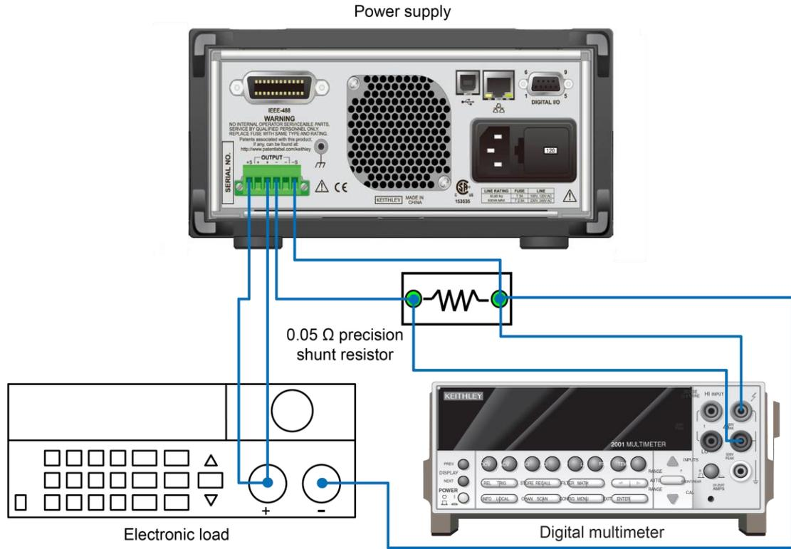
Figure 118: Low-current calibration connection using a resistor
