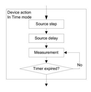
Figure 73: Device action in time mode
