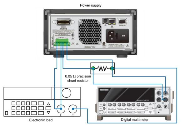
Figure 117: High-current calibration connection using an electronic load
