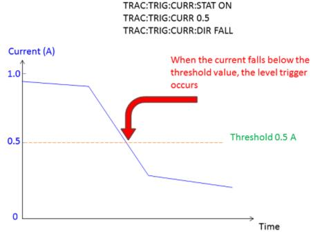
Figure 70: Current level trigger (fall)
