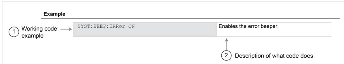
1. Example code that you can copy from this table and paste into your own application. Examples are generally shown using the short forms of the commands.
