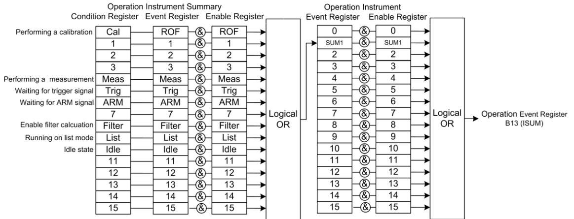
**Figure 122: Status model measurement registers**
