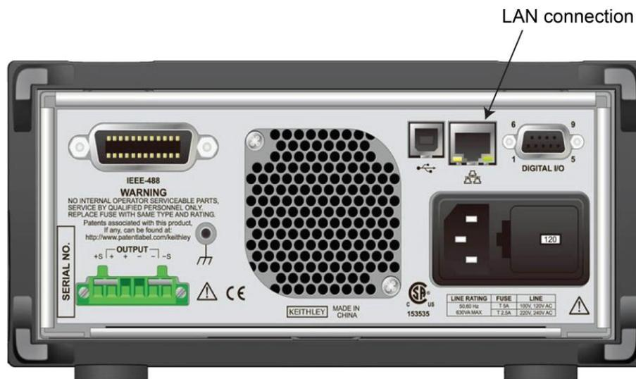
You can connect the instrument to the LAN in a one-to-one, one-to-many, two-network card, or enterprise configuration, as described in the following topics.
