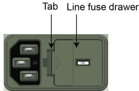
4. Use the screwdriver to lift the tab from the AC receptacle.
