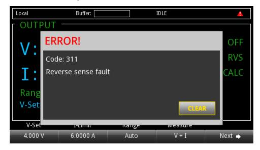
Figure 29: Reversed sense leads error
