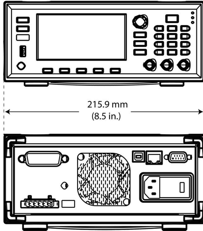
Figure 18: Series 2280 top and side dimensions with bumpers
