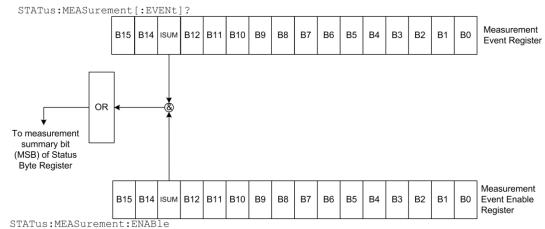
Figure 131: Series 2280 Measurement Event Register
