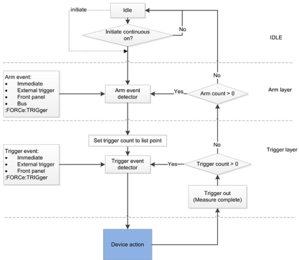
As shown in the previous figure, the device action can be any mode described in [List running time](#) (on page 3-44). The measurement time is set accordingly.
