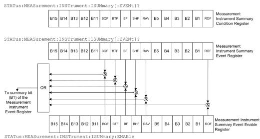
Figure 133: Series 2280 Measurement Instrument Summary Event Register
