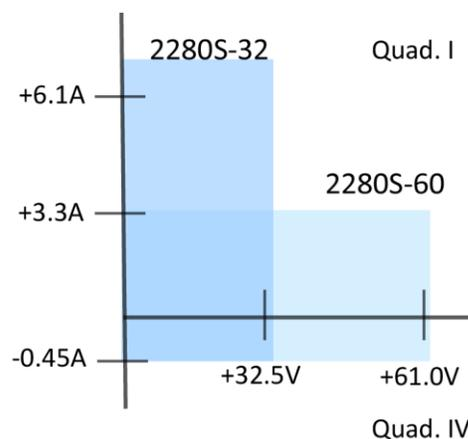
For example, if a 12 V battery is connected to the voltage source (HI to battery high) that is programmed for +10 V, sink operation occurs in the quadrant IV (source +V and measure -I).
