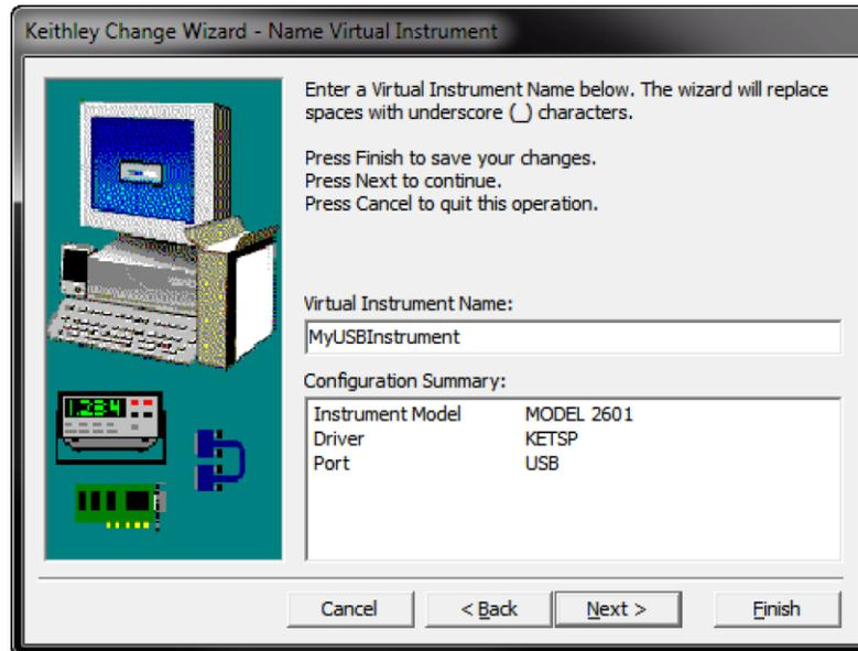
9. In the Virtual Instrument Name box, enter a name that you want to use to refer to the instrument.
