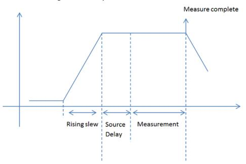
Figure 78: Sweep mode measurement time
