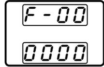
7. Use the current knob to set the Password for the F-00 setting. The Password is "5 0 0 4".
