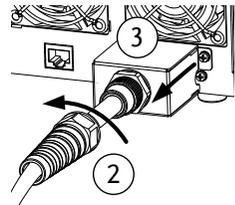
3. Remove the 2 screws holding the power cord cover and remove.
