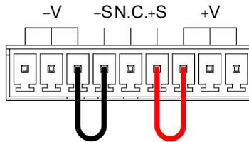
7. If not using local sense, see the remote sense section to wire the sense terminals for remote sensing. Page 71
