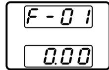
4. Rotate the voltage knob to change the F setting to F-00.
