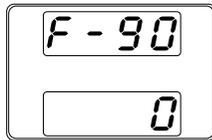
3. Rotate the Voltage knob to change the F setting.
