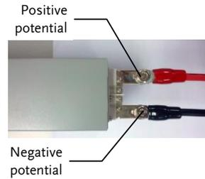
Connection with voltage sense wiring
