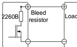
Bleed resistors are designed to dissipate the power from the power supply filter capacitors
