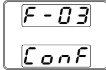
6. If CV Slew Rate Priority was chosen as the operating mode in steps 3~5, set F-04 (Rising Voltage Slew Rate) and F-05 (Falling Voltage Slew Rate) and save.
