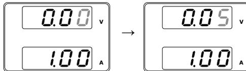
6. Repeatedly press the Voltage knob until the first digit is highlighted. This will allow the voltage to be edited in 1 volt steps.
