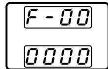
6. Use the current knob to set the Password for the F-00 setting. The Password is "5 0 0 4".
