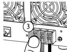
4. Screw the power cord cover onto the rear panel using the supplied screws.
