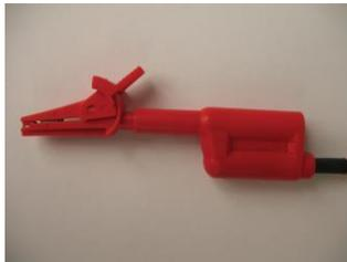
For small cells and electrodes, you can use commercially available banana-to-microclip connectors by plugging them directly into the cable connectors.
