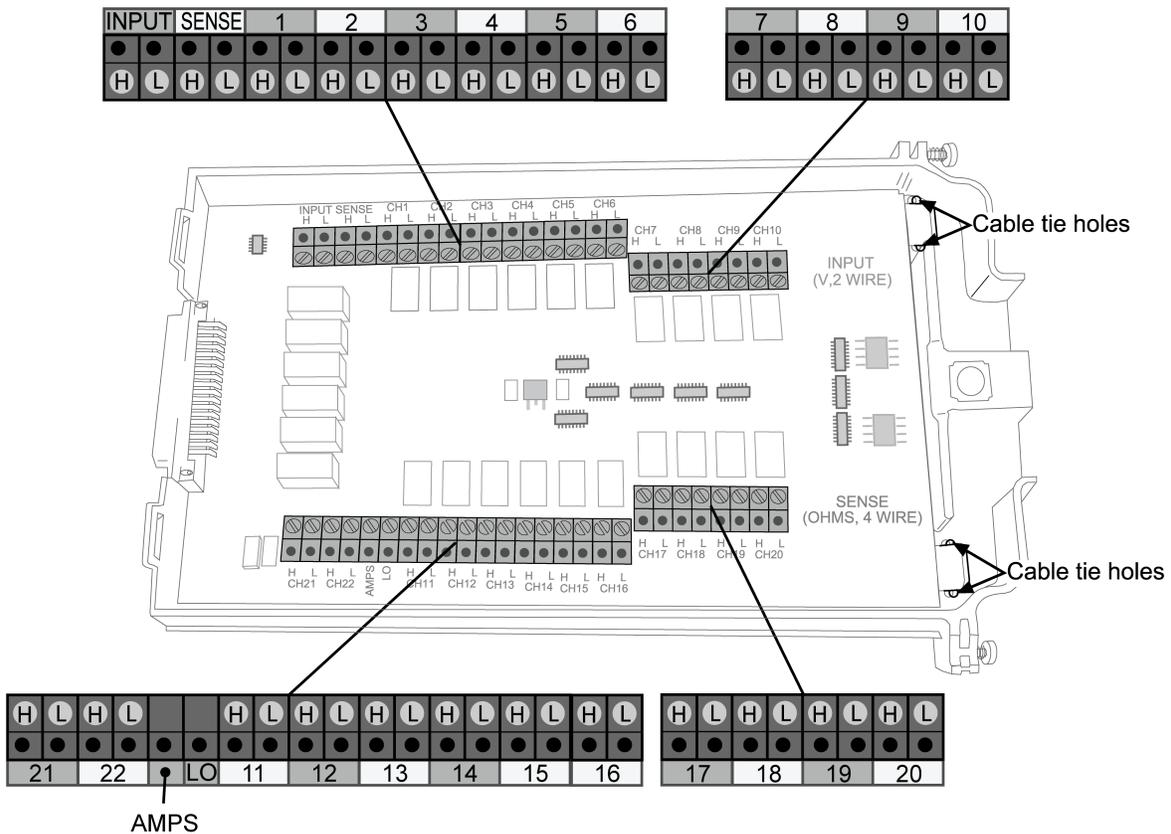
4. Route wire along the wire path and secure with cable tie as shown. The next figure also shows connections to channels 1 and 2.
