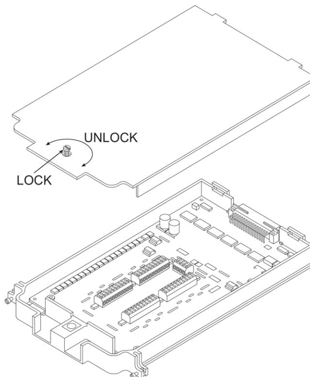
3. If needed, remove the appropriate quick-disconnect terminal block from the module.
