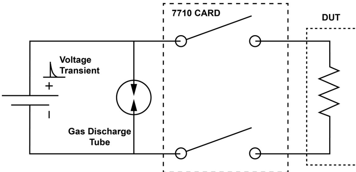
If the device under test (DUT) changes impedance states during testing, excessive currents or voltages may appear at the solid state relay. If a DUT fails due to low impedance, current limiting may be required. If a DUT fails due to high impedance, voltage clamping may be required.
