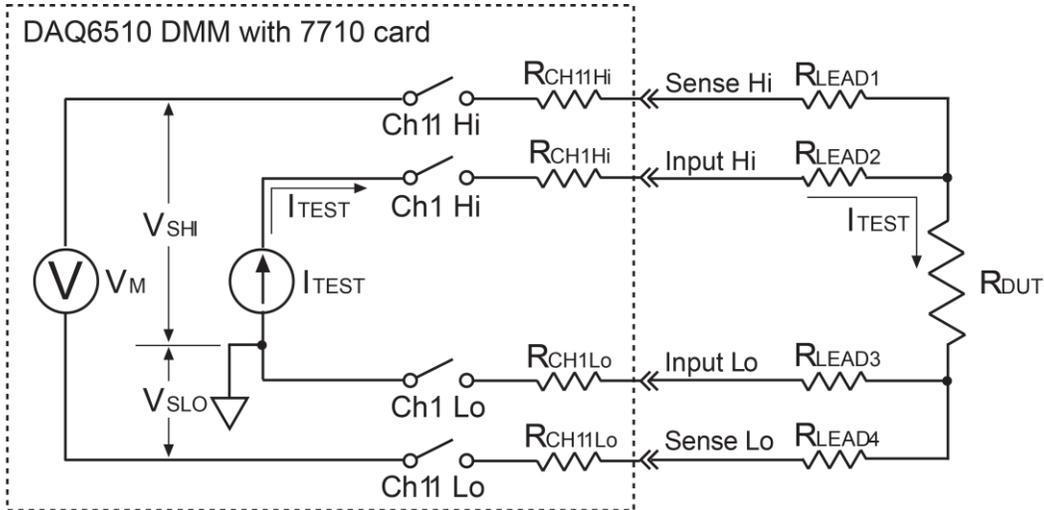
Assumptions: Virtually no current flows in the high-impedance sense circuit due to the high impedance of the voltmeter ( $V_M$ ). Therefore, the voltage drops across Channel 11 and test leads 1 and 4 are negligible and can be ignored.
