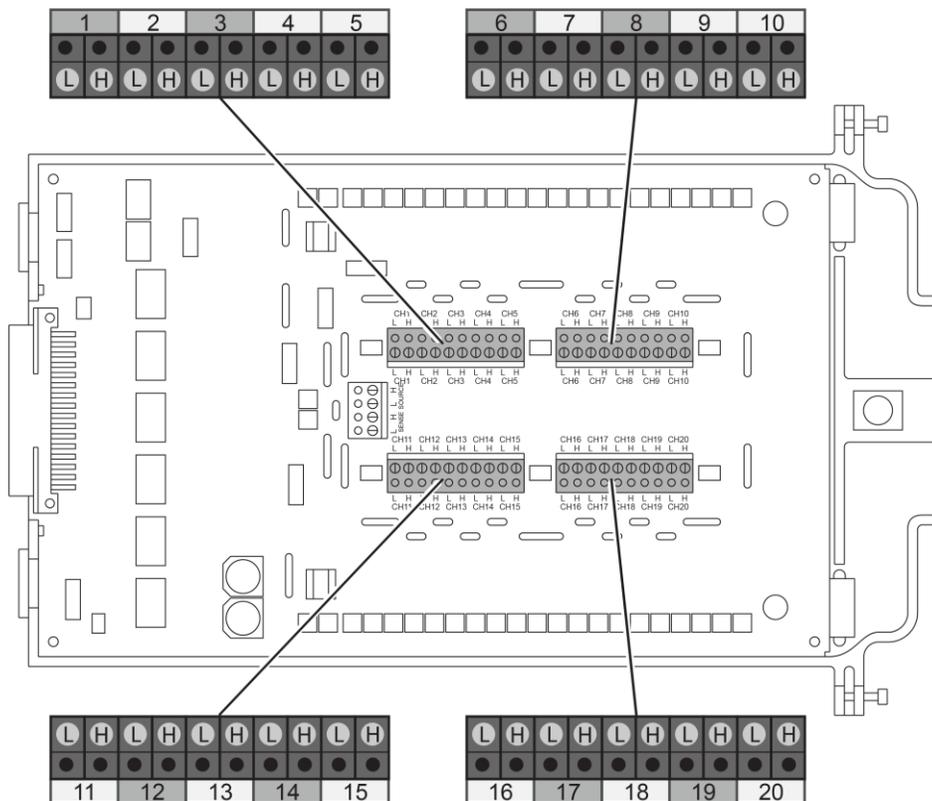
5. Plug the terminal block into the module.
