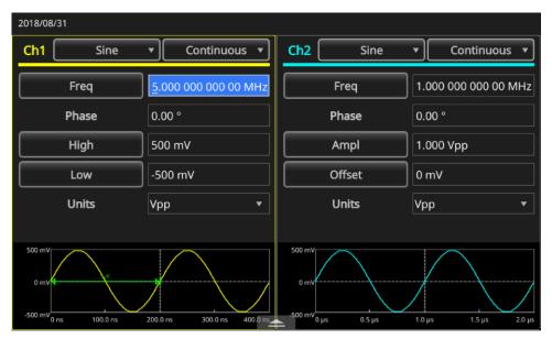
Figure 45: CH1 frequency 5 MHz
