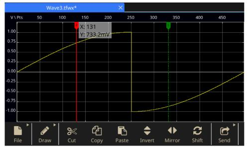
2. Mirror. It is used to overturn the waveform between the cursors in the horizontal direction.
