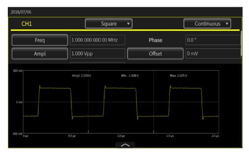
Figure 71: CH1 oscilloscope 1 M $\Omega$  - InstaView
