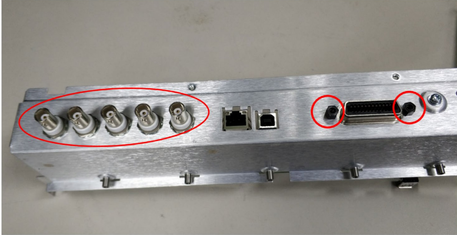
Figure 30: Remove the BNC nuts and GPIB hex screws.
