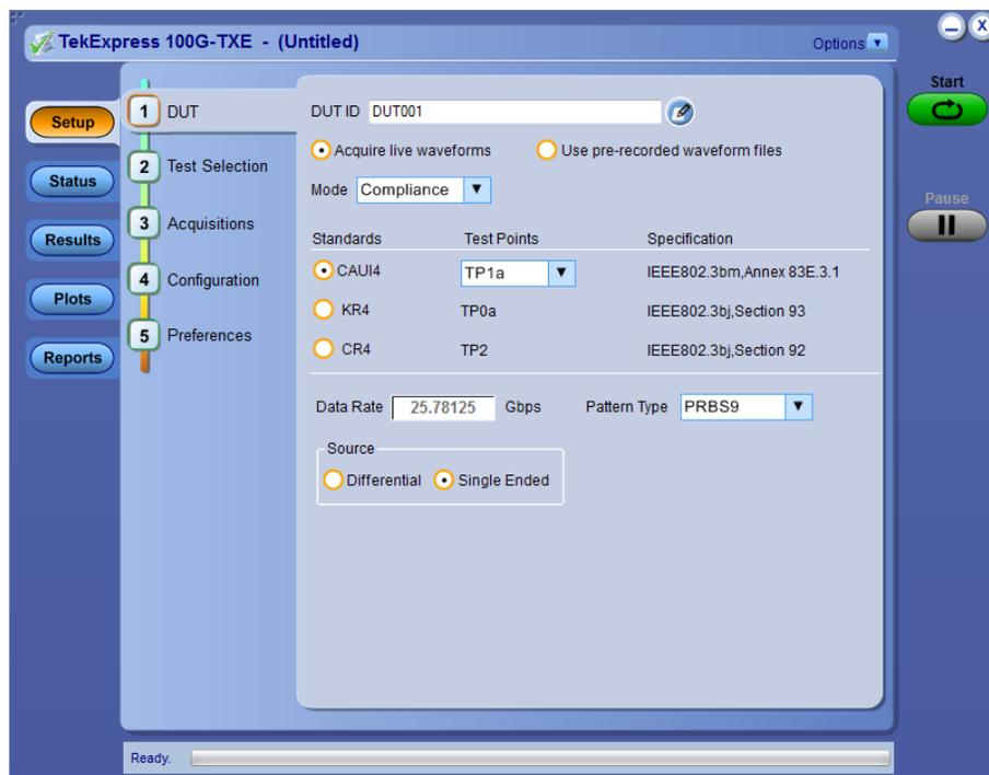
Welcome to the Tektronix 100G-TXE, an Tektronix oscilloscope application software that addresses 100GBASE-CR4, 100GBASE-KR4, and CAUI-4 standards of IEEE. These three electrical standards make up the backbone of the current 100G Ethernet industry, and the TekExpress 100G-TXE automation test solution facilitates turnkey electrical transmitter validation of most 100G Ethernet systems today.
