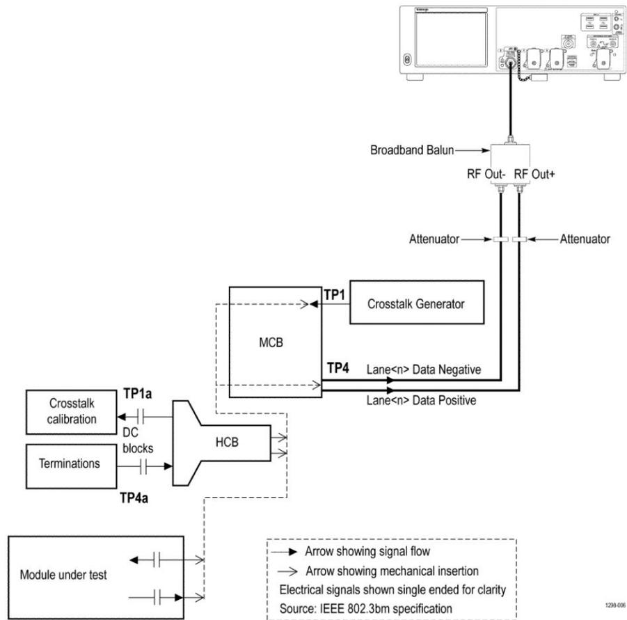
Figure 12: CAUI4 Eye Width / Eye Height TP4 (Differential)
