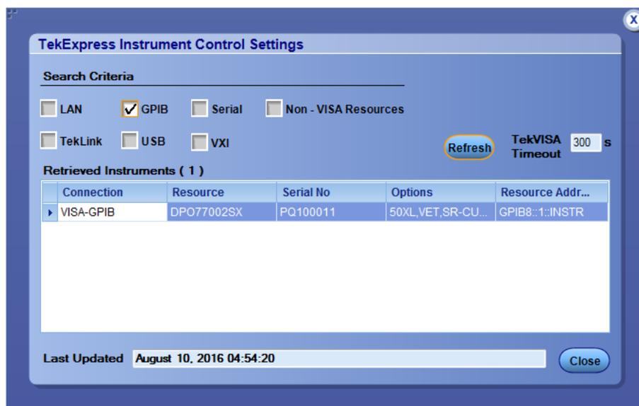
The connected instruments displayed here can be selected for use under Global Settings in the test configuration section.
