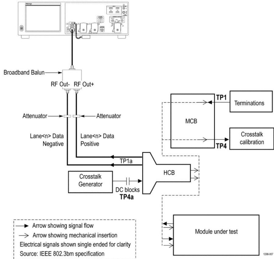
Figure 10: CAUI4 Eye Width / Eye Height TP1a (Differential)
