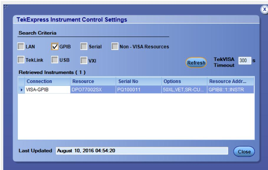
The details of the instruments are displayed in the Retrieved Instruments table. The time and date of instrument refresh is displayed in the Last Updated field.
