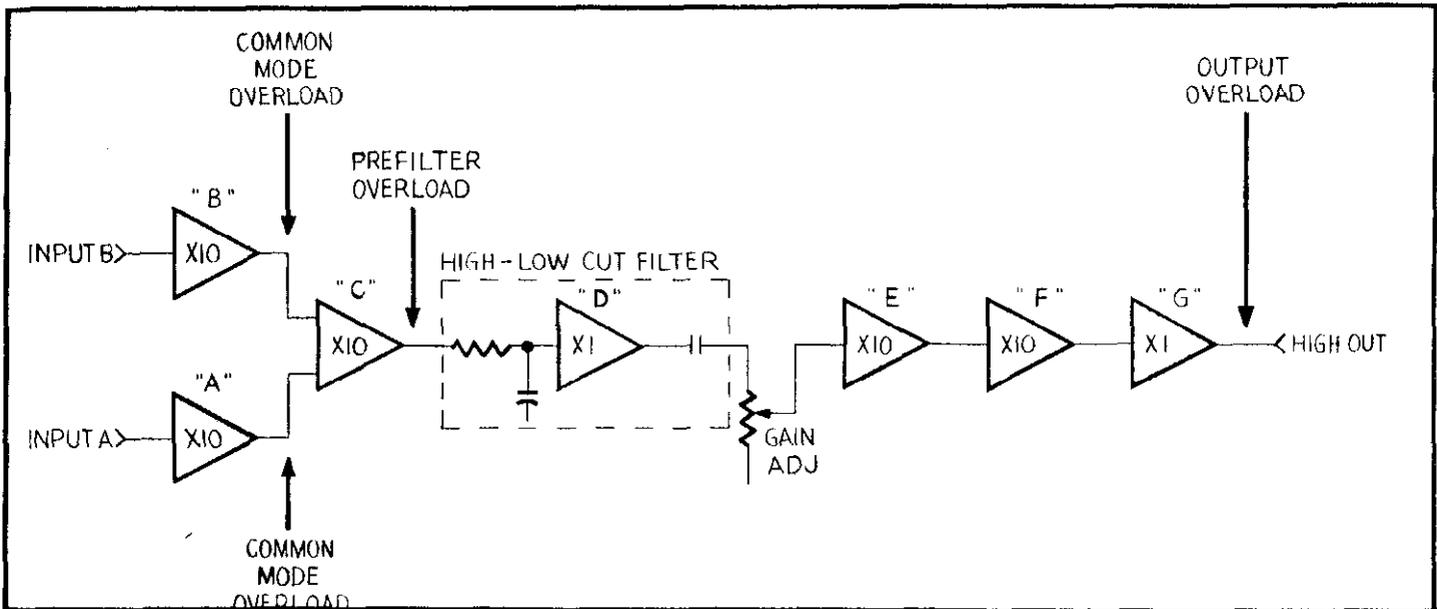
FIGURE 18. Overall Block Diagram.
