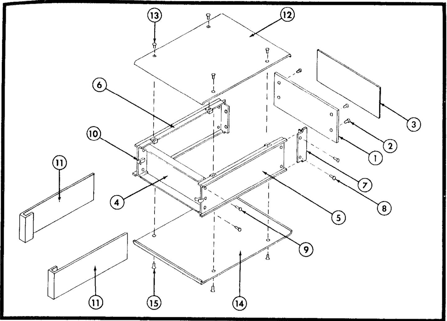
FIGURE 33. Chassis Assembly - Exploded View.
