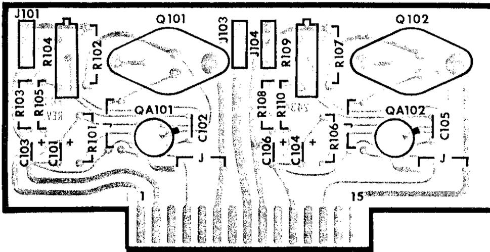
FIGURE 31. Component Layout, PC-261 (Model 1031A Regulator)
