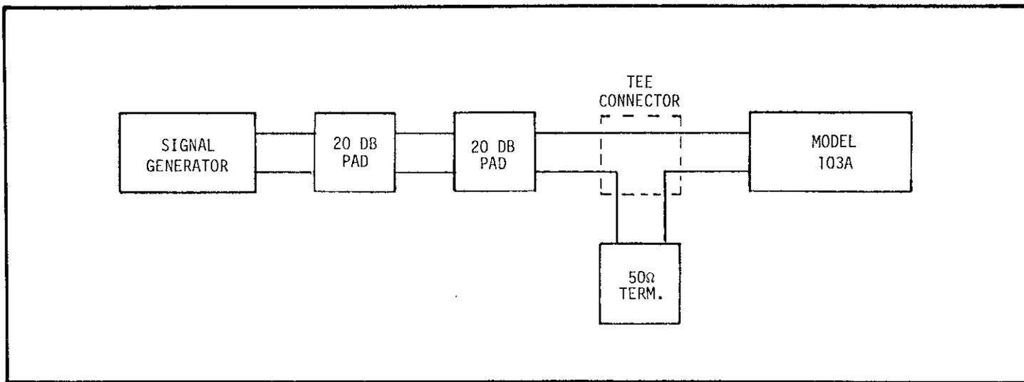
FIGURE 32. Test Set-up for Frequency Response Check.
