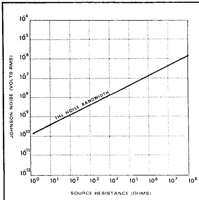
FIGURE 8. Johnson Noise/ $\sqrt{B}$  Versus Source Resistance.
