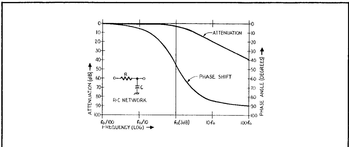
FIGURE 9. Gain/Phase Vs. Frequency For R-C Type Filter.
