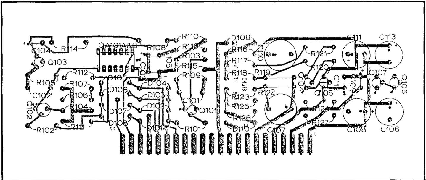
FIGURE 28. Component Layout, PC-293.
