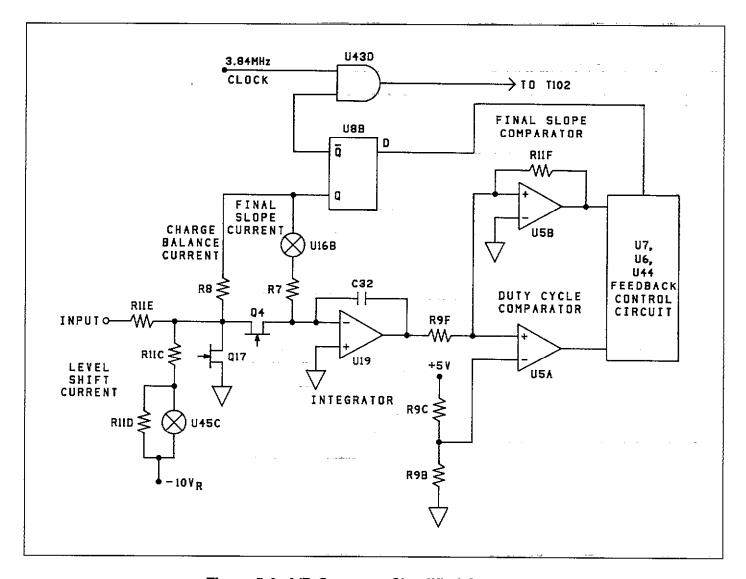
Figure 5-6. A/D Converter Simplified Schematic
