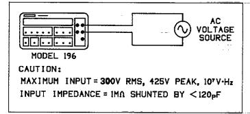
Figure 2-6. TRMS AC Voltage Measurement
