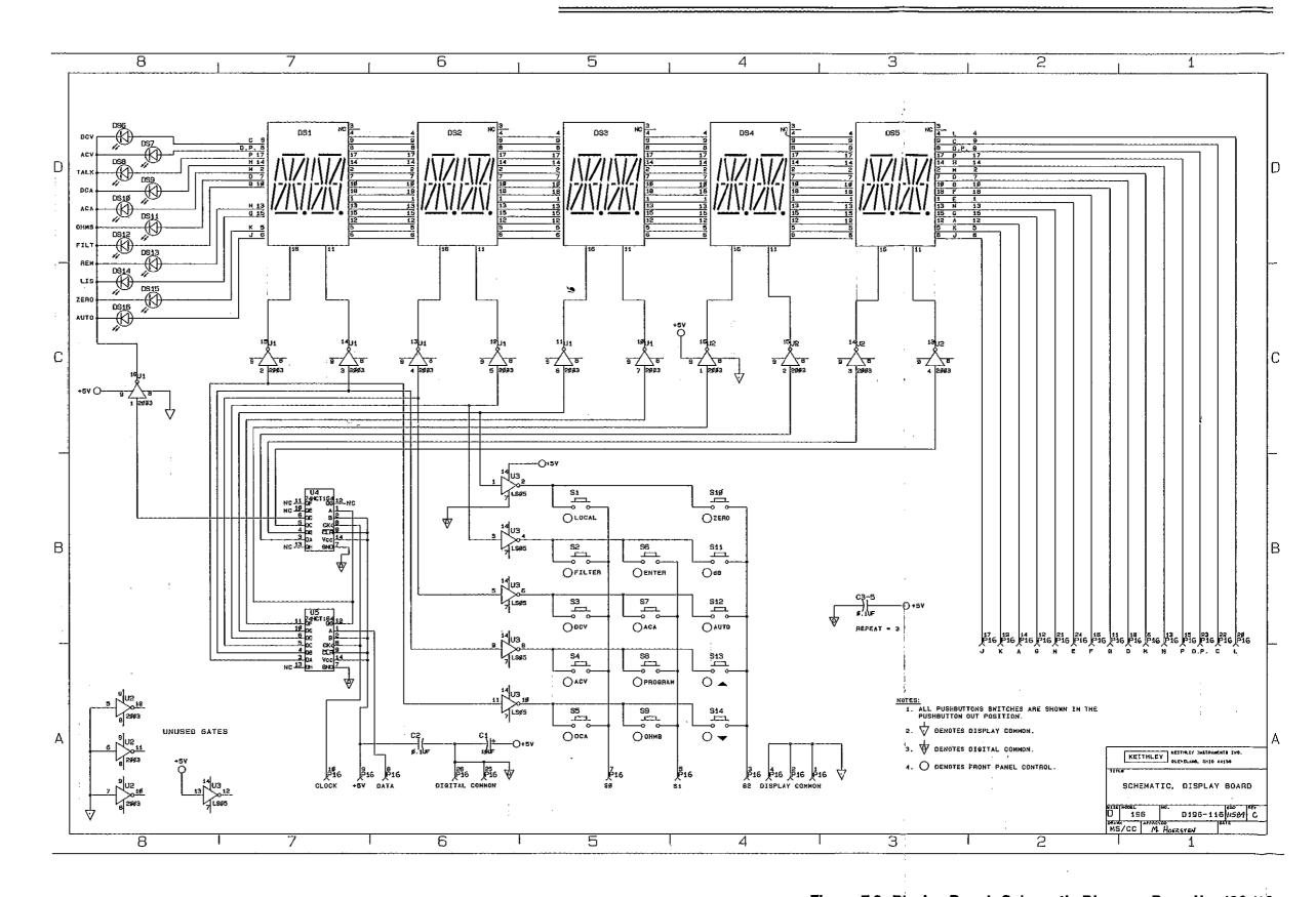
Figure 7-2. Display Board, Schematic Diagram, Dwg. No. 196-116
