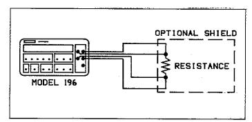
Figure 2-5. Four-Terminal Resistance Measurements
