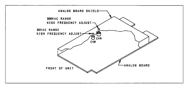
Figure 6-7. TRMS AC Volts High Frequency Calibration Adjustments (30V & 300V Ranges)
