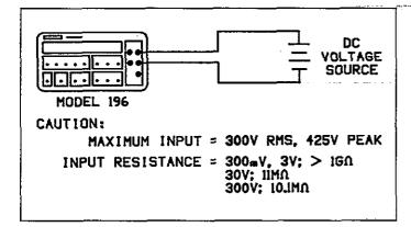
Figure 2-3. DC Voltage Measurements
