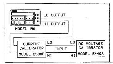
2. Connect the AC current calibration source to the Model 196 as shown in Figure 4-6.
