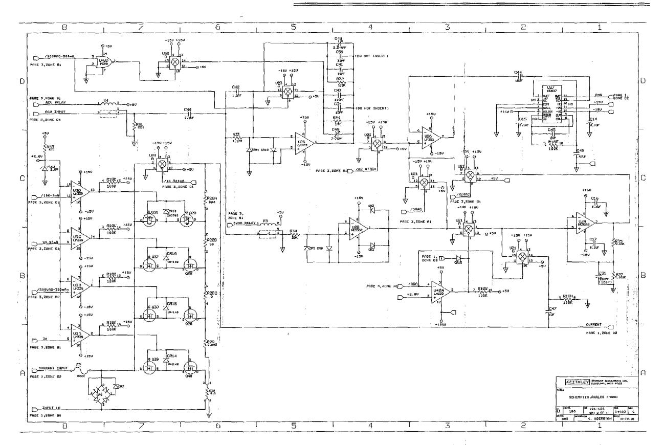
Figure 7-6. Analog Board, Schematic Diagram, Dwg. No. 196-126 (sheet 2 of 4)
