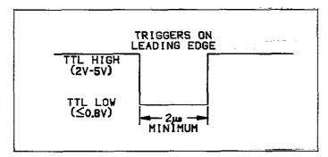
Figure 2-8. External Trigger Pulse Specifications
