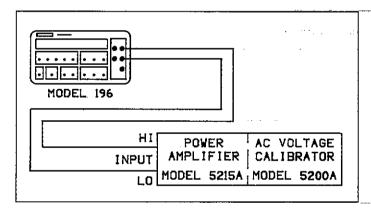
Figure 4-2. Connections for TRMS AC Volts Verification
