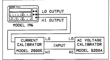
Figure 4-6. Connections for TRMS AC Current Verification
