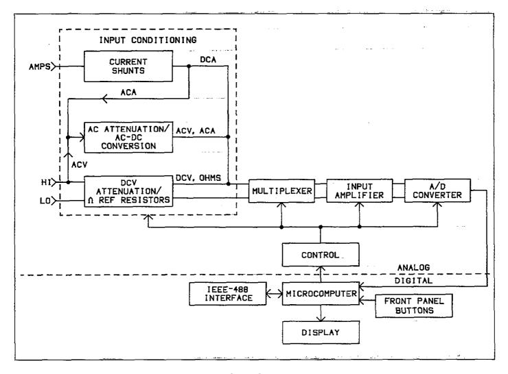
Figure 5-1. Overall Block Diagram
