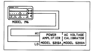
Figure 6-6. TRMS AC Volts Calibration Configuration
