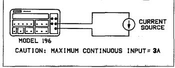
Figure 2-7. Current Measurements
