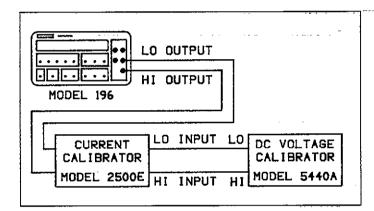
Figure 6-8. DC Current Calibration Configuration
