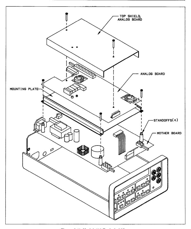
Figure 6-11. Model 196 Exploded View
