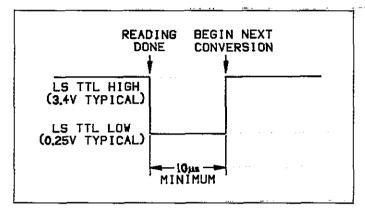
Figure 2-9. Voltmeter Complete Pulse Specifications
