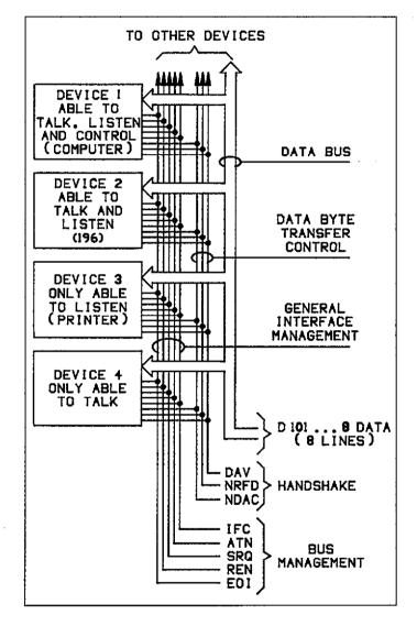
Figure D-1. IEEE Bus Configuration
