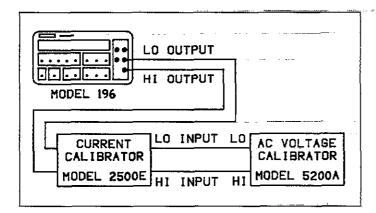
Figure 6-9. AC Current Calibration Configuration
