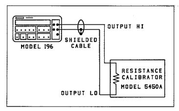
Figure 4-4. Connections for Ohms Verification (300k $\Omega$ —300M $\Omega$  Ranges)
