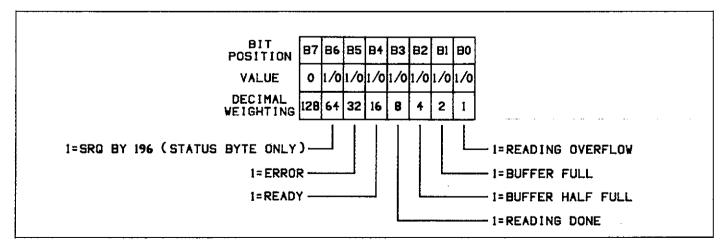
Figure 3-7. SRQ Mask and Serial Poll Byte Format
