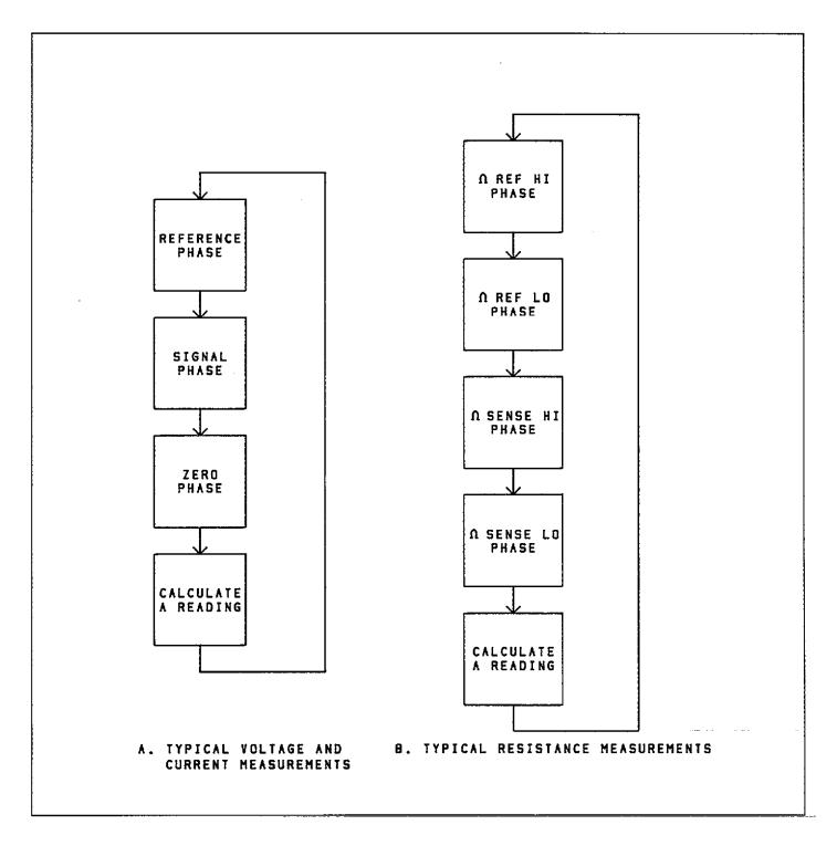
Figure 5-5. Mutliplexer Phases
