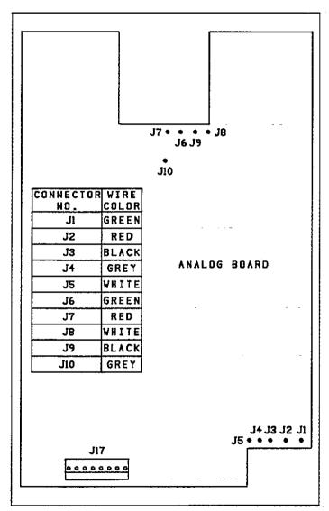
Figure 6-10 Analog Board Connectors
