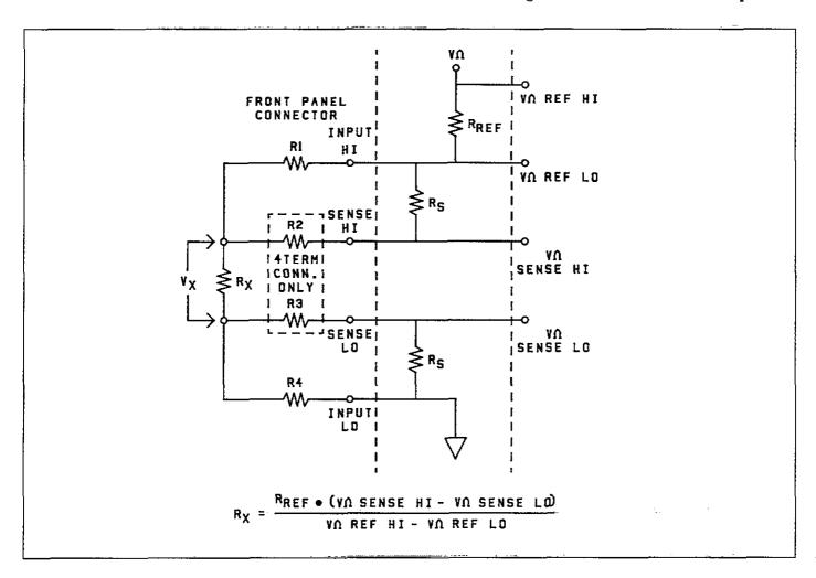
Figure 5-2. Input Configuration During 2 and 4-Terminal Resistance Measurement
