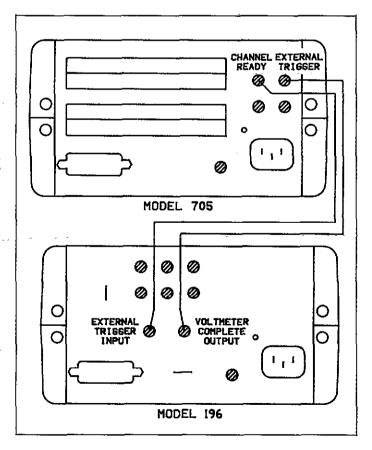
Figure 2-10. External Triggering Example
