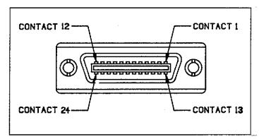
Figure 3-5. Contact Assignments
