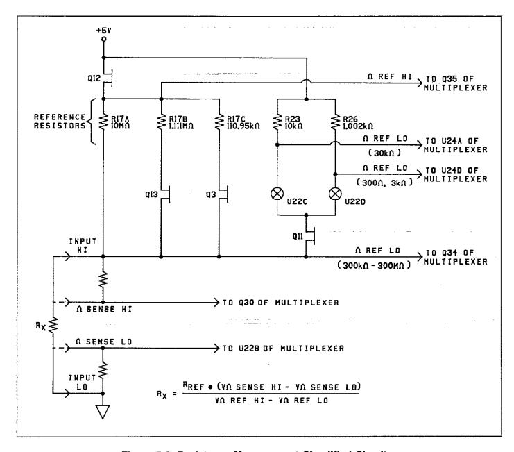
Figure 5-3. Resistance Measurement Simplified Circuitry
