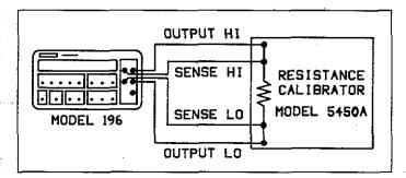
Figure 6-3. Four-Wire Resistance Calibration Configuration (300Ω-30kΩ Ranges)
