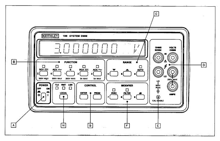
Figure 2-1. Model 196 Front Panel
