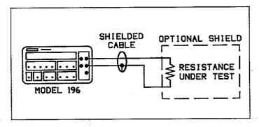
Figure 2-4. Two-Terminal Resistance Measurements
