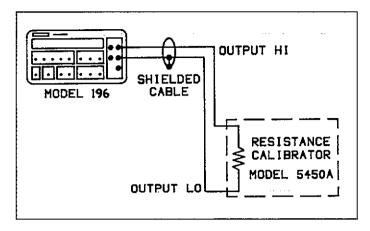
Figure 6-4. Two-Wire Resistance Calibration Configuration (300k $\Omega$ -300M $\Omega$  Ranges)
